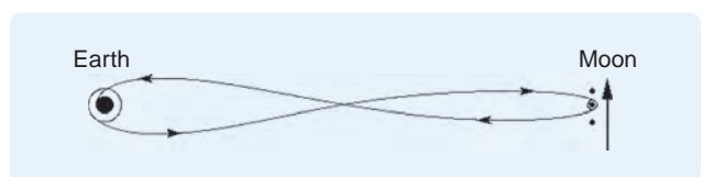
FIGURE 1 Nominal Apollo trajectories, drawn approximately to scale in nonrotating coordinates. The trajectory control problem is further complicated by the orbital velocity of the Moon around the Earth at about 1 km/s. The Moon completes nearly a quarter of its orbit around the Earth during the mission to the Moon and back.
