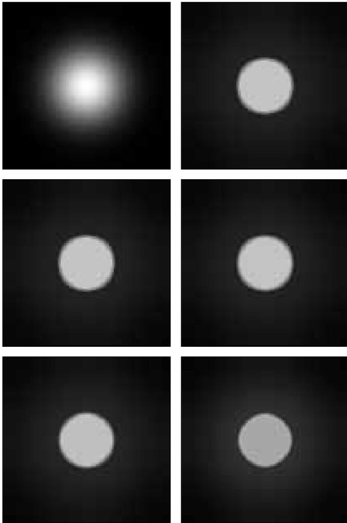
Fig. 1. Nonlinear diffusion filtering of a Gaussian-like test image ( $\lambda = 8$ ,  $\sigma = 1.5$ ). (a) TOP LEFT: Original image,  $\Omega = (0, 101)^2$ . (b) TOP RIGHT: Explicit scheme, 800 iterations,  $\tau = 0.25$ . (c) MIDDLE LEFT: AOS scheme, 800 iterations,  $\tau = 0.25$ . (d) MIDDLE RIGHT: AOS scheme, 200 iterations,  $\tau = 1$ . (e) BOTTOM LEFT: AOS scheme, 40 iterations,  $\tau = 5$ . (f) BOTTOM RIGHT: AOS scheme, 10 iterations,  $\tau = 20$ .
