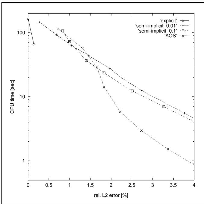
Fig. 3. Tradeoff between efficiency and accuracy of nonlinear diffusion solvers. The data were calculated on the test image from Fig. 2, size  $\Omega = (0, 255) \times (0, 308)$ . Filter parameters:  $\lambda = 2$ ,  $\sigma = 1$ . Stopping time:  $T = 200$ . Hardware: one R10000 processor on an SGI Challenge XL.
