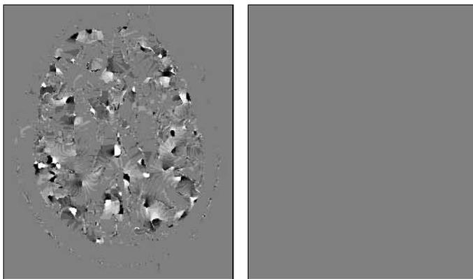
Fig. 4. (Non-)Commutation of nonlinear diffusion operators. The difference between filtering prior to rotation by 90 degrees, and rotation prior to filtering is depicted. Test image: Figure 2 ( $\lambda = 2$ ,  $\sigma = 1$ ,  $\tau = 20$ , 10 iterations). (a) LEFT: A multiplicative splitting such as LOD treats x and y axes differently. (b) RIGHT: Additive operator splitting (AOS) treats all axes equally.
