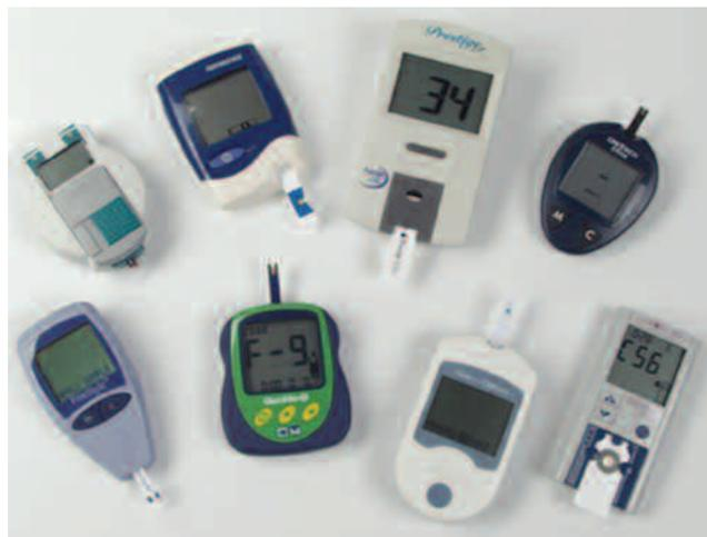
With the 21st century came a number of different electrochemical glucose meter systems, including the OneTouch Ultra (top right) from Johnson & Johnson.
