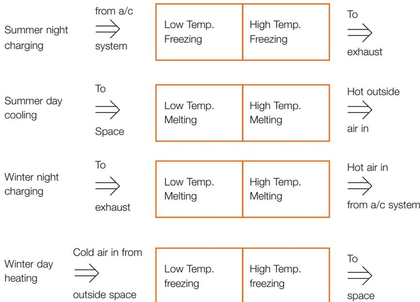
Figure 1 - night time charging and day time utilisation process during both heating and cooling seasons for a reverse cycle refrigerative heat pump system.
