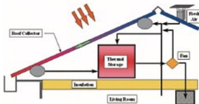
Figure 2 - schematic of the solar heating system
