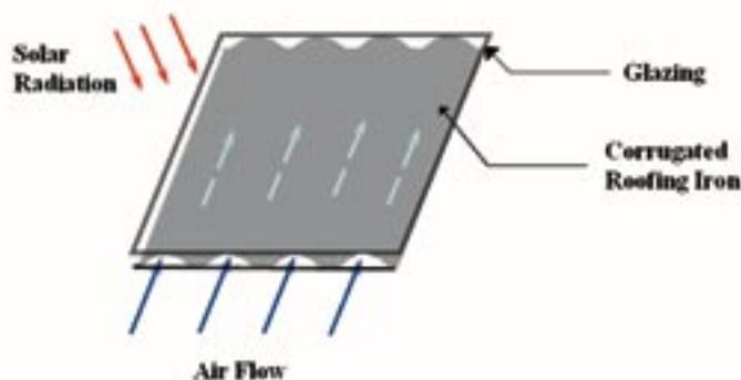
Figure 3 - roof-integrated collector
