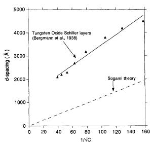
Figure 4. Schiller layer *d*-spacing for tungsten oxide platelets measured as a function of NaCl concentration. The broken line denotes the predicted *d*-spacing of the Sogami theory from Equation [4].
