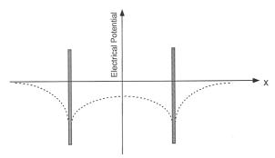
Figure 2. Electrostatic attraction (Sogami) model of electrical potential as a function of distance, x, between 2 clay plates.
