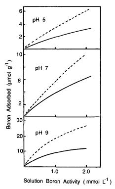
Figure 5. Boron adsorption isotherms for pyrophyllite at 3 pH values and 2 electrolyte concentrations, 0.01 *M* NaNO<sub>3</sub> (solid lines) and 0.1 *M* NaNO<sub>3</sub> (broken lines). Figure adapted from Keren and Sparks (1994).
