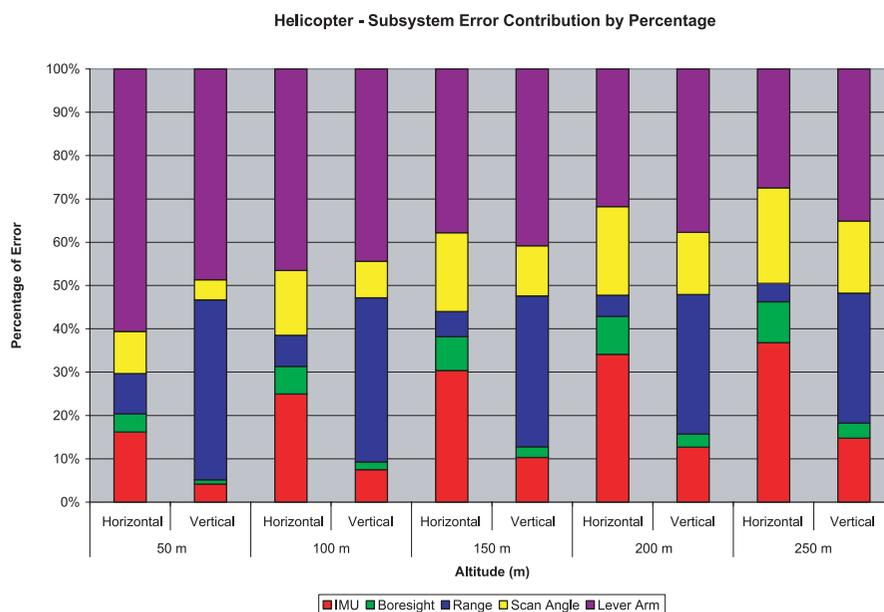
Figure 7: Helicopter, Subsystem Error Contribution by Percentage (Applanix 510 IMU, Q-280 Laser)
