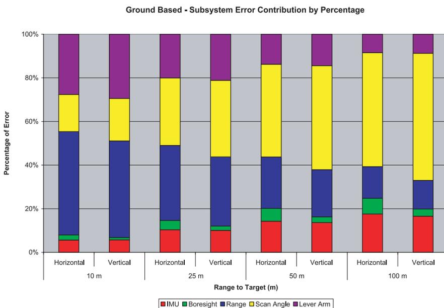
Figure 9: Ground System, Subsystem Error Contribution by Percentage (510 IMU, LSQ Boresight, 0.5 cm Lever Arm Error)
