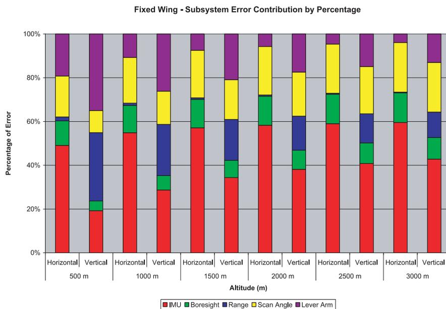
Figure 4: Fixed Wing System, Subsystem Error Contribution by Percentage (Applanix 510 IMU, Least Squares Boresight)
