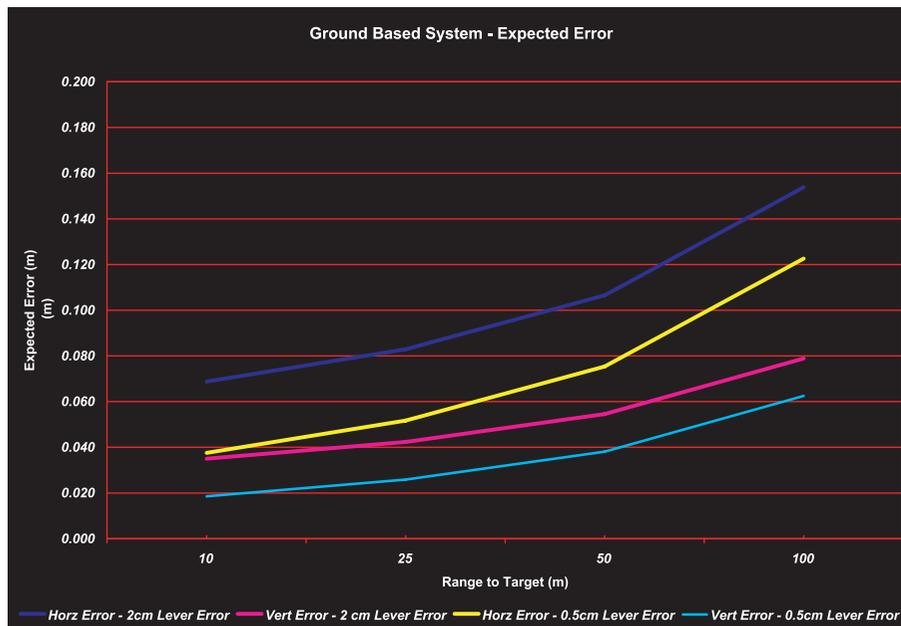
Figure 8: Ground Based System Horizontal and Vertical Errors for Two Different Lever-Arm Errors
