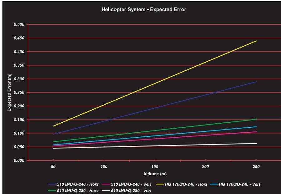
Figure 5: Helicopter System Horizontal and Vertical Errors for Three Different Scenarios
