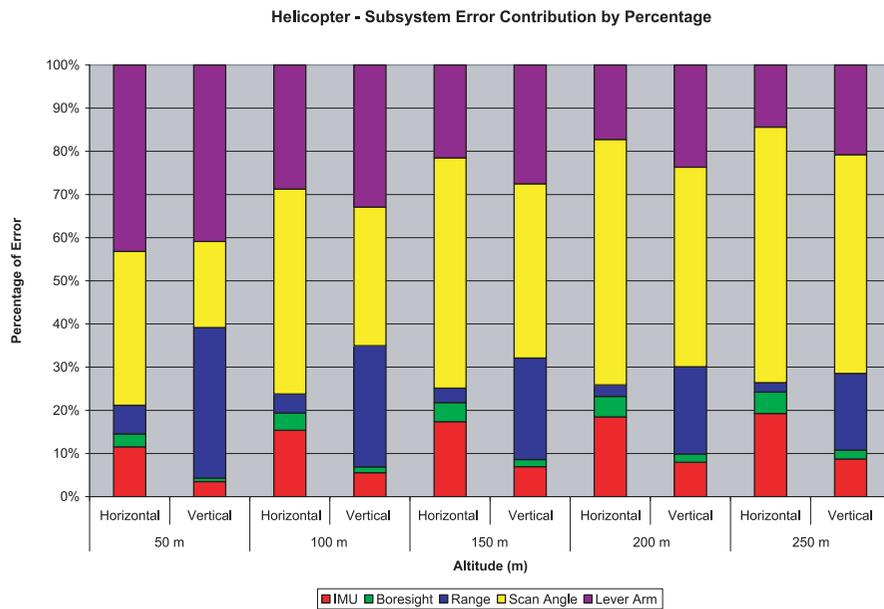
Figure 6: Helicopter, Subsystem Error Contribution by Percentage (Applanix 510 IMU, Q-240 Laser)
