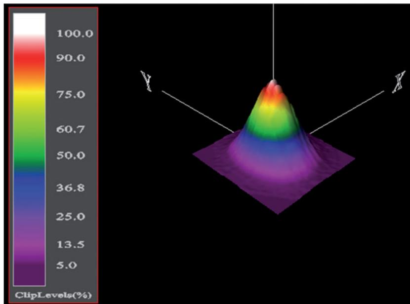
Figure 1: Relative Power Distribution of Output Pulse From Terrapoint ALTM LIDAR System
