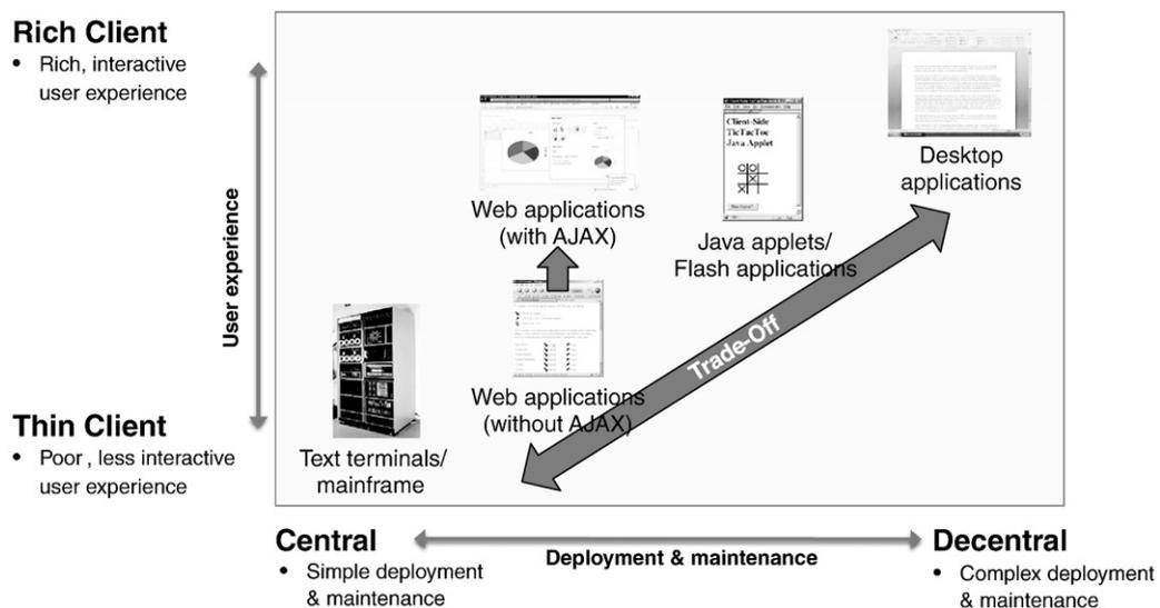
Fig. 2. Web applications break trade-off between rich and thin clients.
