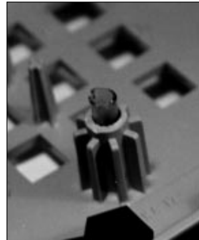
Figure 8: SMP compression sleeve inserted inside injection moulded form bolt acceptor inside the BT telephone
