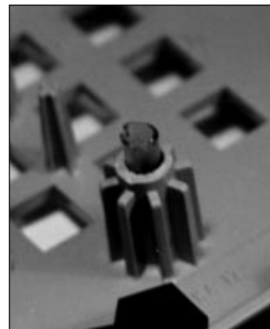
Figure 9: Slightly undersized bolt inserted inside SMP compression sleeve within injection mould assembly bolt acceptor inside the BT telephone
