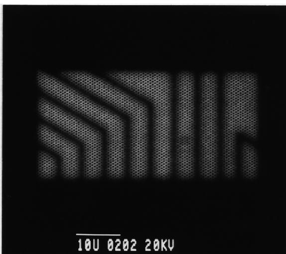
Fig. 1 Top view of formed photonic crystal with defect waveguides
