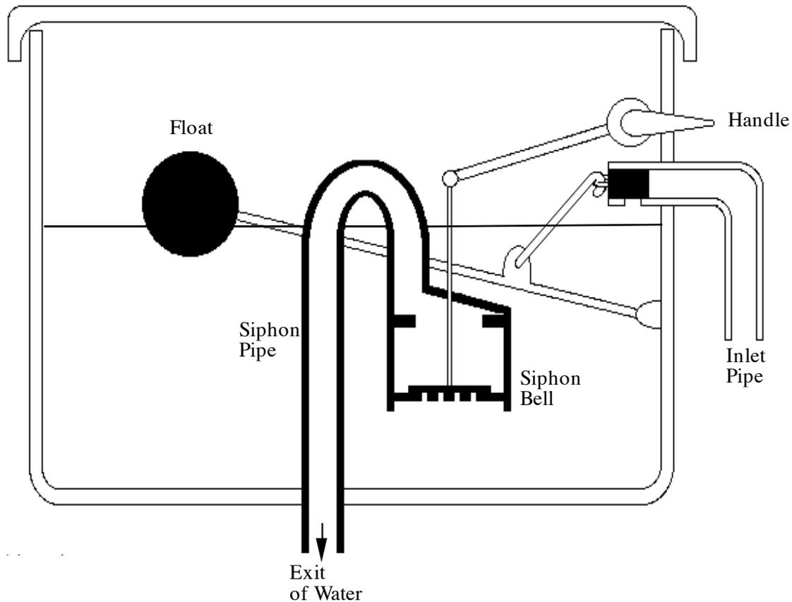
**Figure 1:** A Flushing Cistern
