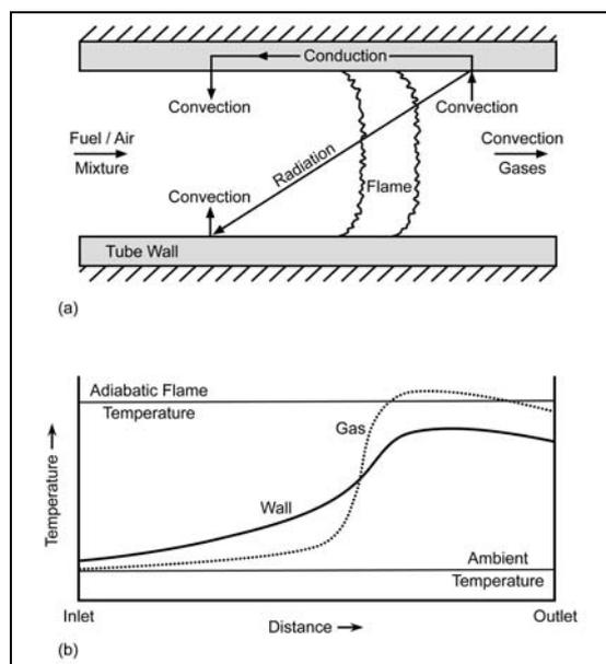
Figure 2 a) Schematic of heat transfer within a tube and b) the corresponding temperature profile (based on<sup>13</sup>)
