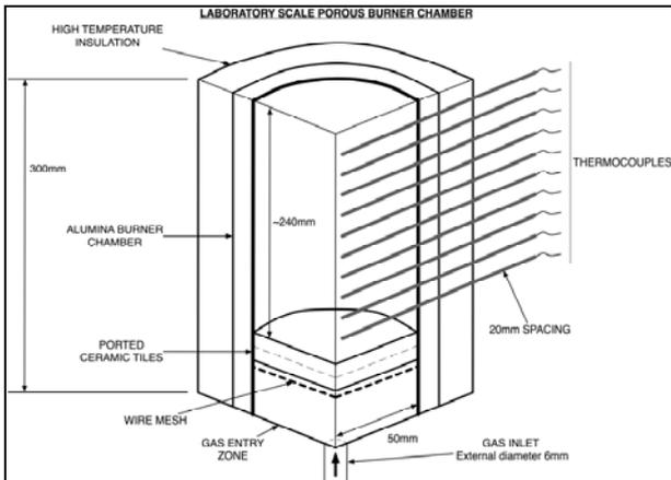
Figure 7 Schematic of the porous burner chamber, with no porous media shown for clarity
