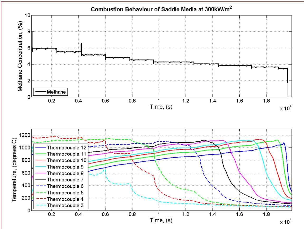
Figure 10 Typical experimental output for one media type at 300kW/m<sup>2</sup> firing rate, uppermost graph showing methane concentration over time and lower graph showing corresponding temperature profile
