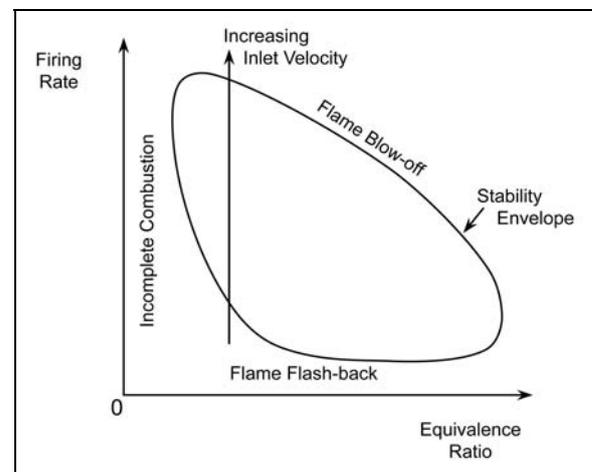
Figure 3 Burner stability envelope (based on<sup>22</sup>)
