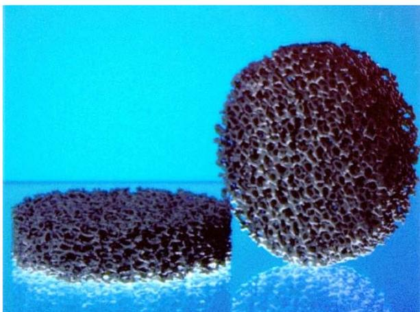
Figure 5 Silicon carbide open-cell foam<sup>9</sup>
