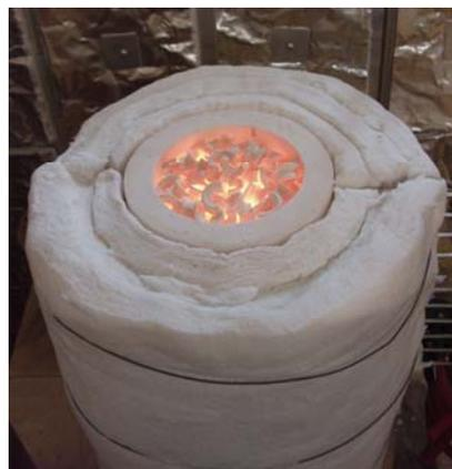
Figure 1 The heated surface of a volumetric porous burner.
