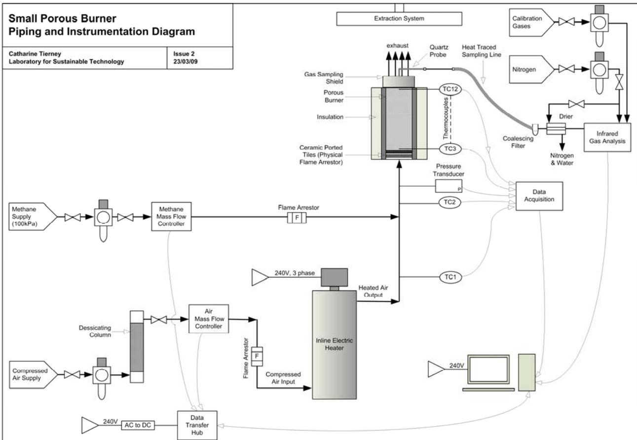
Figure 8 Piping and instrumentation diagram for the laboratory porous burner system
