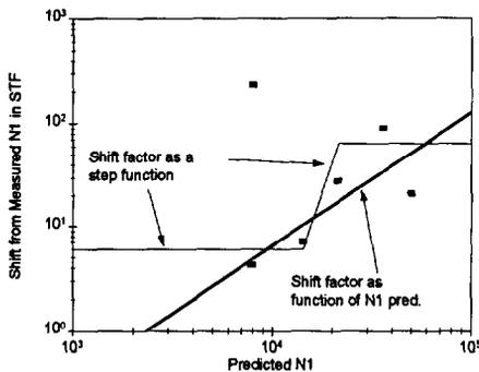
**Figure 23: Shift factor as a Step Function or as a Function of Predicted N1**
