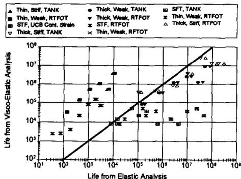
**Figure 27: Comparison of Various Structures, Elastic versus Visco\_Elastic Analysis, Mix AAG-RD**
