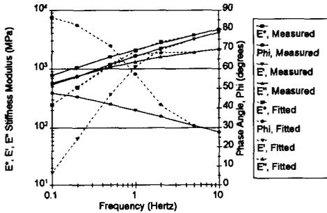
**Figure 13: Complex Properties Measured and Fitted with Two Maxwell Elements in Parallel**
