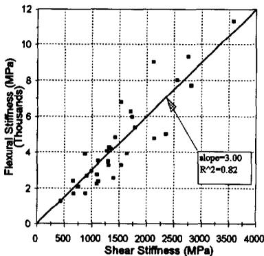
**Figure 16: Relationship Between Shear and Flexural Stiffness**
