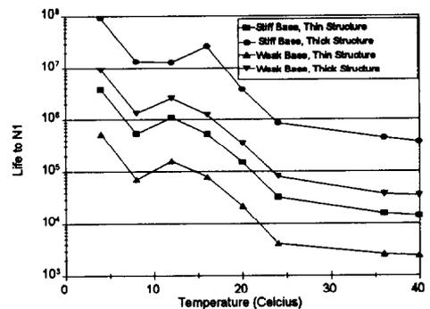
Figure 26: Predicted Life using Visco-Elastic Analysis for Thick and Thin Pavement Structures on Weak and Strong Bases
