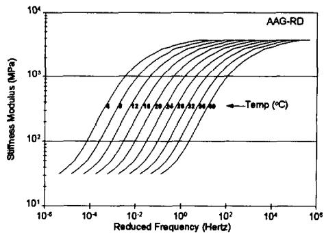
**Figure 18: Complex Stiffness Modulus for Mix AAG-RD between 4°C and 40°C**
