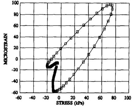
Figure 7: Calculated Longitudinal Hysteresis Loop at underside of bound layer
