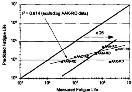
**Figure 22: Calculated vs. Observed Results for the Slab Experiments**
