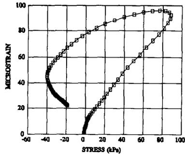
Figure 8: Calculated Transverse Hysteresis Loop at underside of bound layer
