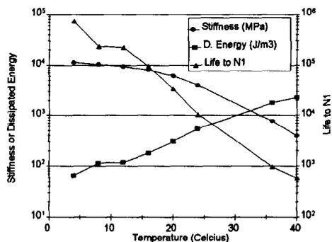
**Figure 24: Results from Visco-elastic Analysis of the Slab Mix AAG-RD**
