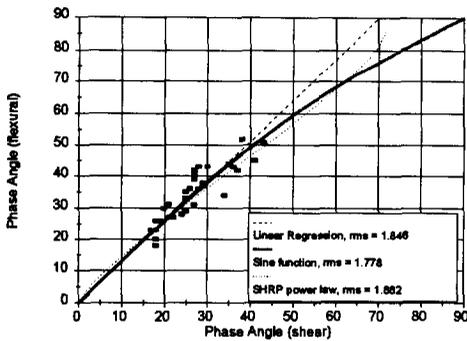
**Figure 15: Phase Angle Measurements, Flexural vs. Shear**
