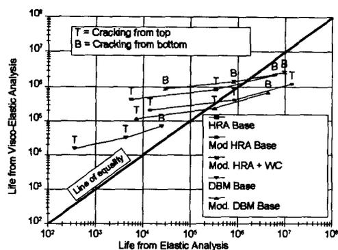
**Figure 31: Comparison of Results Between Elastic and Visco-Elastic Analysis**
