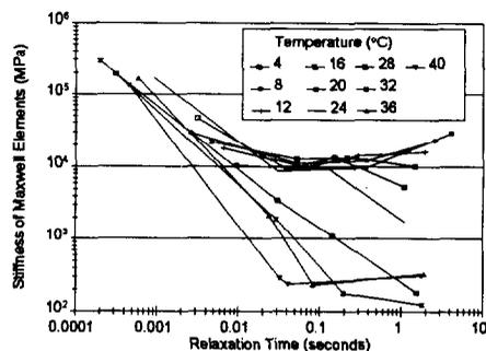
**Figure 19: Discrete Relaxation Spectrum for Various Temperatures for Mix AAG-RD**
