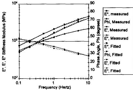
**Figure 14: Complex Properties Measured and Fitted with Four Maxwell Elements in Parallel**
