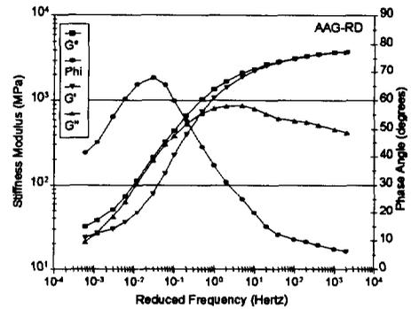
**Figure 17: Master Curve Reduced to 20°C for Mixture AAG-RD in Simple Shear**
