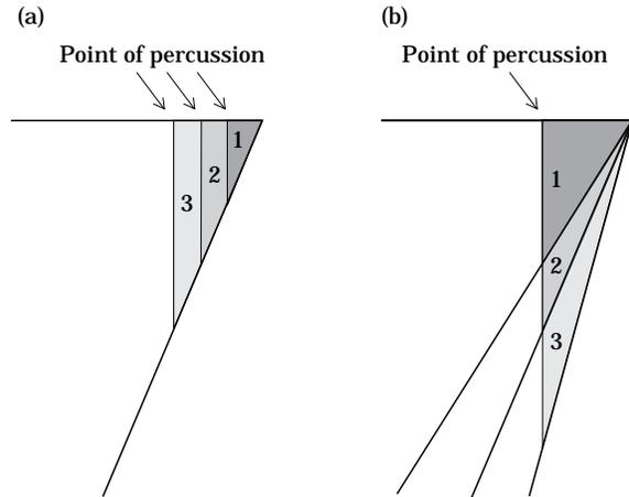
Figure 3. Comparison of the changes in volume of material removed with increases in (a) exterior platform angle or (b) platform depth.
