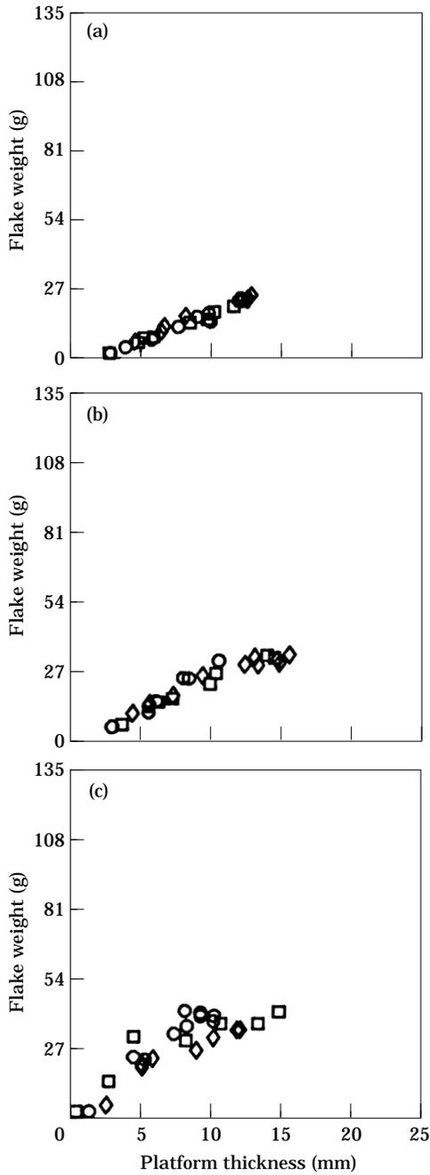
Figure 5. Graph of platform thickness versus weight for a constant momentum (1500), but varying velocity (drop height) and indenter mass. Momentum is held constant by dropping the lighter balls from increased height, thereby increasing their velocities. Exterior platform angle: (a) 55°; (b) 65°; (c) 75°. ○, 0.34 m drop height and 224 g ballbearing weight; □, 1.71 m and 45 g; ◇, 2.75 m and 28 g.
