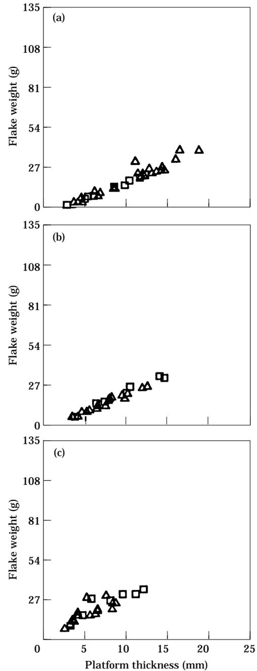
Figure 6. Graph of platform thickness versus weight for the 45 g ball bearing dropped from two different heights: △, 1.25 m; □, 1.71 m. Exterior platform angle: (a) 55°; (b) 65°; (c) 75°. Note that the corresponding changes in velocity and momentum for a constant mass do not affect the mass of the flake.
