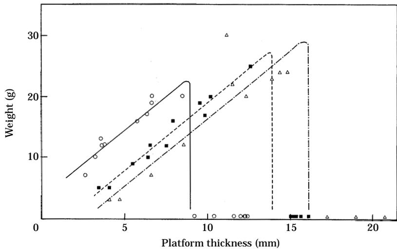
Figure 11. Graph of the platform thickness versus weight for the 45 g ball dropped from 1.25 m. Flakes with a weight of 0 g are incipient cones formed at platform thicknesses which are too great for the amount of momentum applied to the core. Note that as the exterior platform angle increases so the value of platform thickness which produces a flake decreases:  $\Delta$  and  $-\cdot-\cdot$ , 55°;  $\blacksquare$  and  $----$ , 65°;  $\circ$  and  $—$ , 75°.
