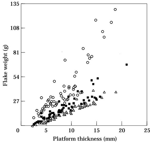
Figure 2. Graph of platform thickness versus flake weight for all flakes, including all combinations of indenter mass and velocity. Exterior platform angles:  $\circ$ , 75°;  $\blacksquare$ , 65°,  $\triangle$ , 55°.
