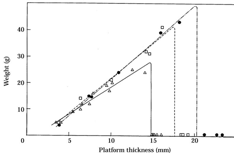
Figure 12. Graph of the platform thickness versus weight for the 45 g ball dropped from three different heights with cores having exterior platform angles of 65°:  $\triangle$  and —, 1.25 m;  $\square$  and - - - -, 1.75 m;  $\bullet$  and - . - ., 2.15 m. As the velocity of the ball is increased, so does the maximum value of the platform thickness which can produce a flake.
