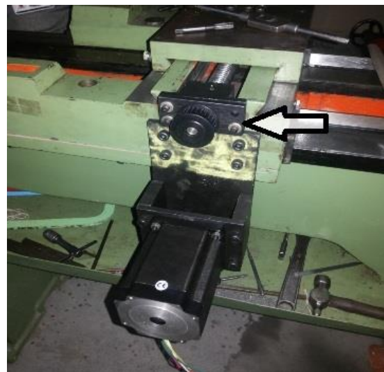
Fig. 9 X-axis mounting & stepper motor
