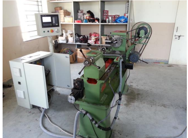
Fig. 12 Developed retrofitted lathe machine
