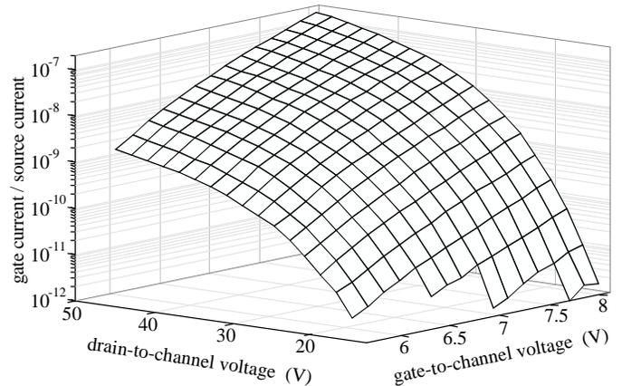
Fig. 7. Synapse-transistor injection efficiency versus drain-to-channel and gate-to-channel voltages. The RMS deviation between these data and Eqn. (5) is  $1.2 \times 10^{-9}$ .
