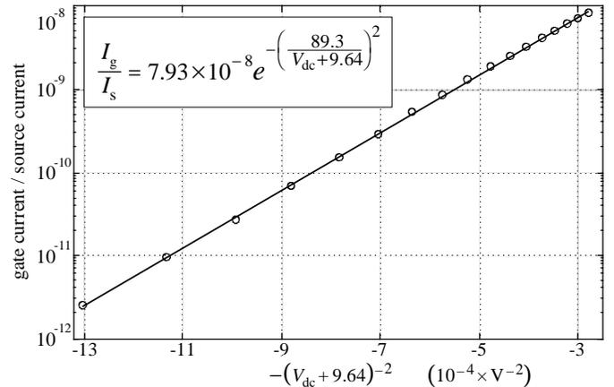
Fig. 5. Synapse-transistor CHEI efficiency versus drain-to-channel voltage, for  $V_{gc}=6.7\text{V}$  and  $I_s=2\mu\text{A}$ .
