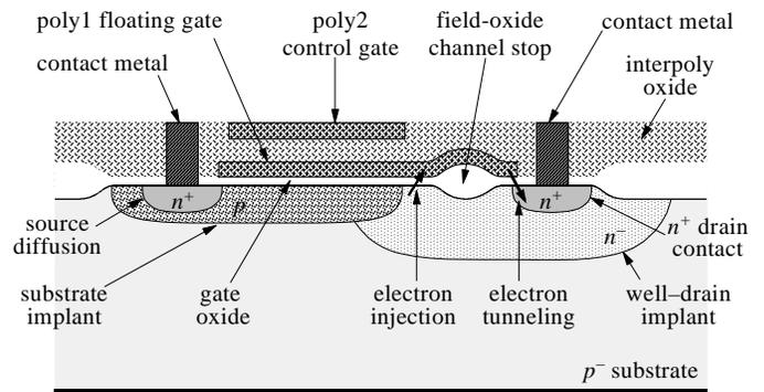
Fig. 2. Synapse transistor, side view, showing the tunneling and injection locations. As a consequence of the  $p$ -type substrate implant, the floating-gate to channel-surface coupling coefficient,  $\kappa$ , is 0.2.
