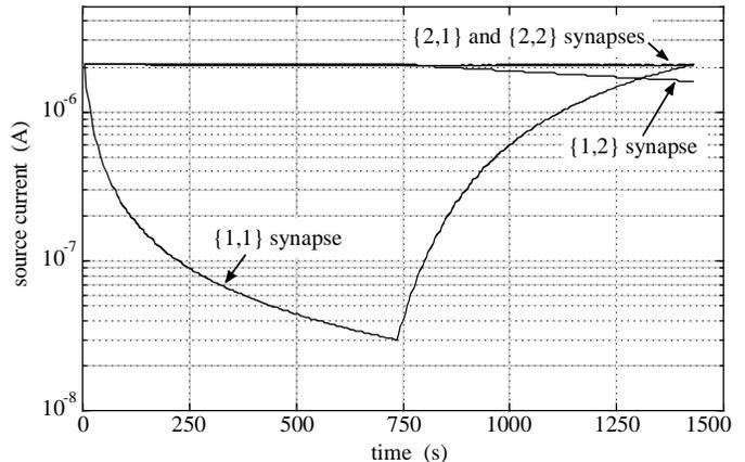
Fig. 12. Isolation in a  $2 \times 2$  synaptic array. Source current is the synapse output. The  $\{1,1\}$  synapse first is injected down to 30 nA, then is tunneled back up to  $2 \mu\text{A}$ . Crosstalk to the  $\{1,2\}$  synapse, defined as the fractional change in the  $\{1,2\}$  synapse divided by the fractional change in the  $\{1,1\}$  synapse, is 0.43%.
