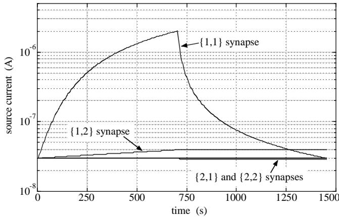
Fig. 13. The same experiment as in Fig. 12, but here the {1,1} synapse first is tunneled up to  $2\mu\text{A}$ , then is injected back down to  $30\text{nA}$ . Crosstalk to the {1,2} synapse is 0.52%.
