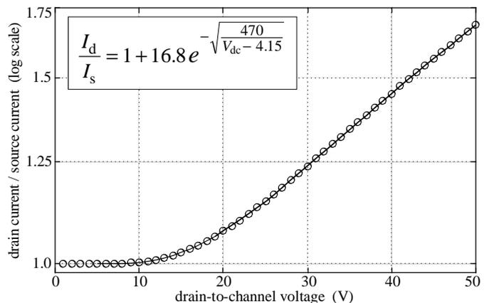
Fig. 8. Synapse-transistor impact ionization versus drain-to-channel voltage, for  $V_{gc}=6.15$  V and  $I_s=100$  nA. The fit function is independent of source current for  $2$  nA  $< I_s < 2$  μA.
