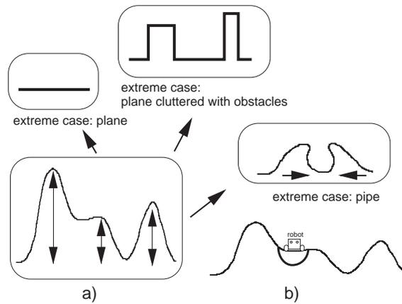
Figure 3: Robot-environment interactions in the Huegellandschaft. *a)* systematically varying the surface by the experimenter *b)* modification of the surface by moving robots, development of trails or ‘building behavior’
