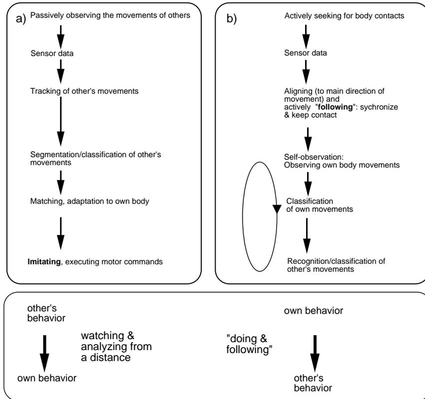
Figure 9: Two different ways of approaching imitation of movements. *a)* ‘traditional approach’, *b)* self-observational approach. The circle indicates a feedback loop, i.e. movement which are pleasurable or displeasing for the imitator can be used to cause interruption of the following behavior. For further explanation, see text.
