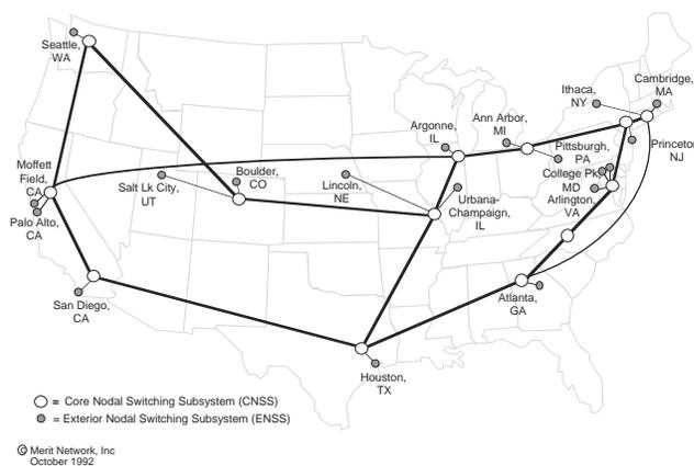
Figure 1: 1992 NSFNET T3 Backbone Service Logical Topology
