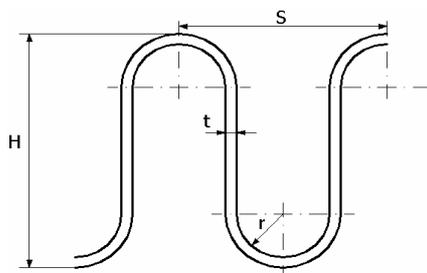
Fig.2 Heating coil element
