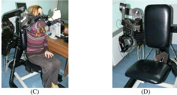
**Figure 3.** The arm exoskeleton during the execution of the reaching task. A: the starting position of the reaching task; B: a subject in the middle of the path of the reaching task; C: a subject at the end-point of the path of the reaching task; D: The overall system.
