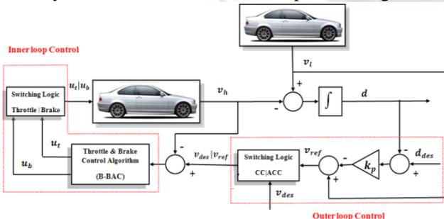
Fig.5 the block diagram of ACC system including inner loop control, the outer loop control and the switching logic from [6]
