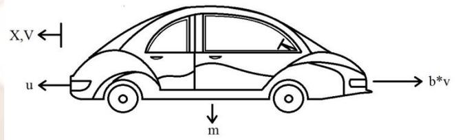
Fig.1. Free-body diagram of a car
