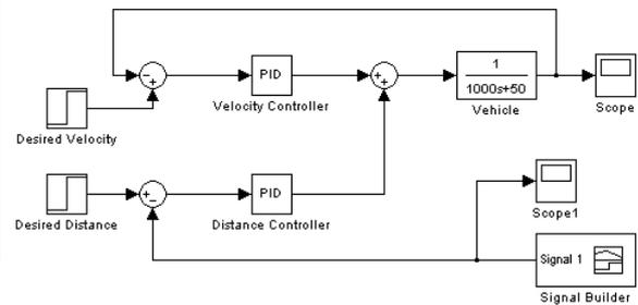
Fig7. A Trial ACC Simulation Model
