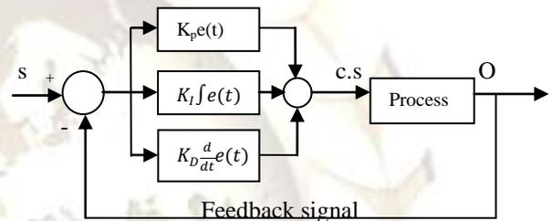
Fig.6 PID Controller
