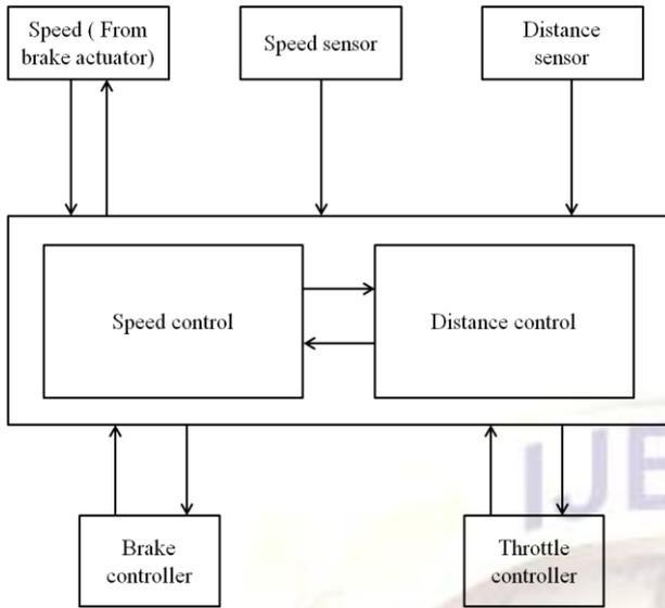
Fig.4 ACC signals and information flow
