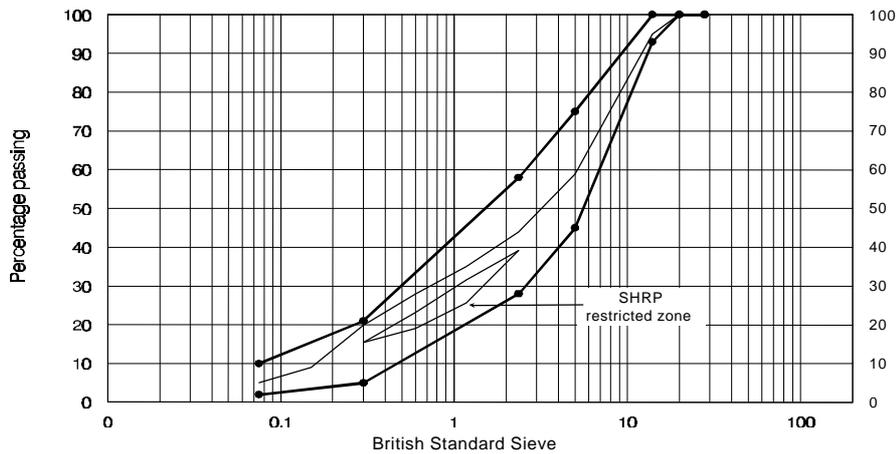
**Figure 2: Grading curve for AC mix**
