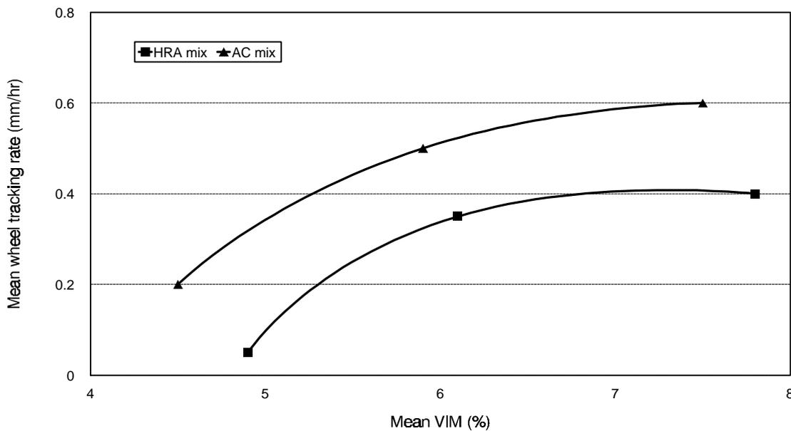
**Figure 6: Relationship between mean VIM and mean wheel tracking rates**
