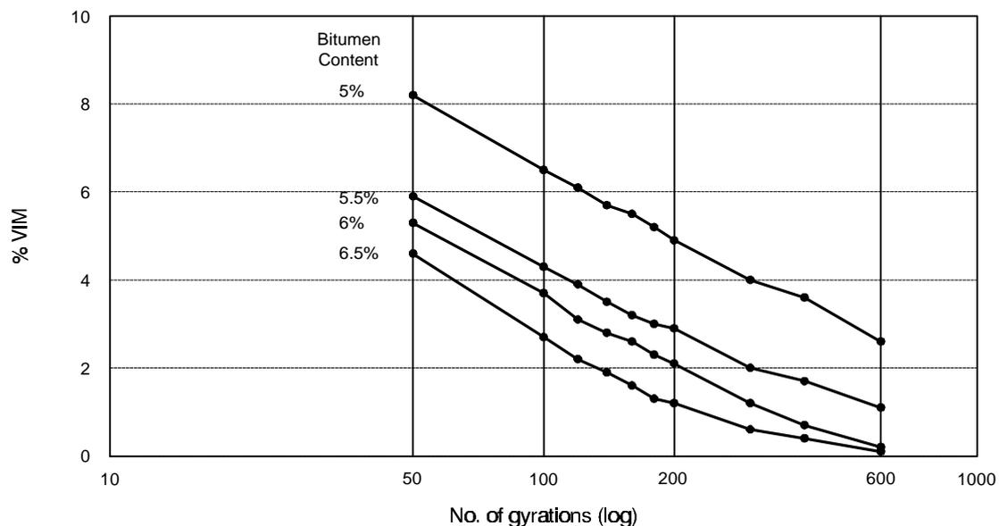
**Figure 4: VIM v Number of gyrations for AC mix**
