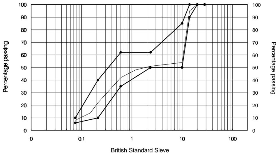
**Figure 3: Grading curve for HRA mix**
