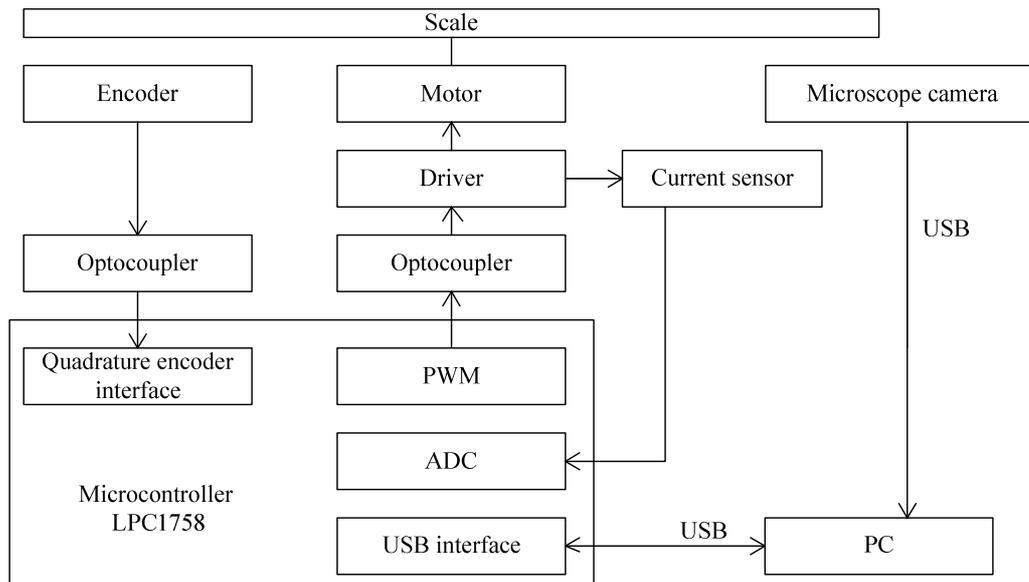
Fig. 2. Functional diagram of modified controller
