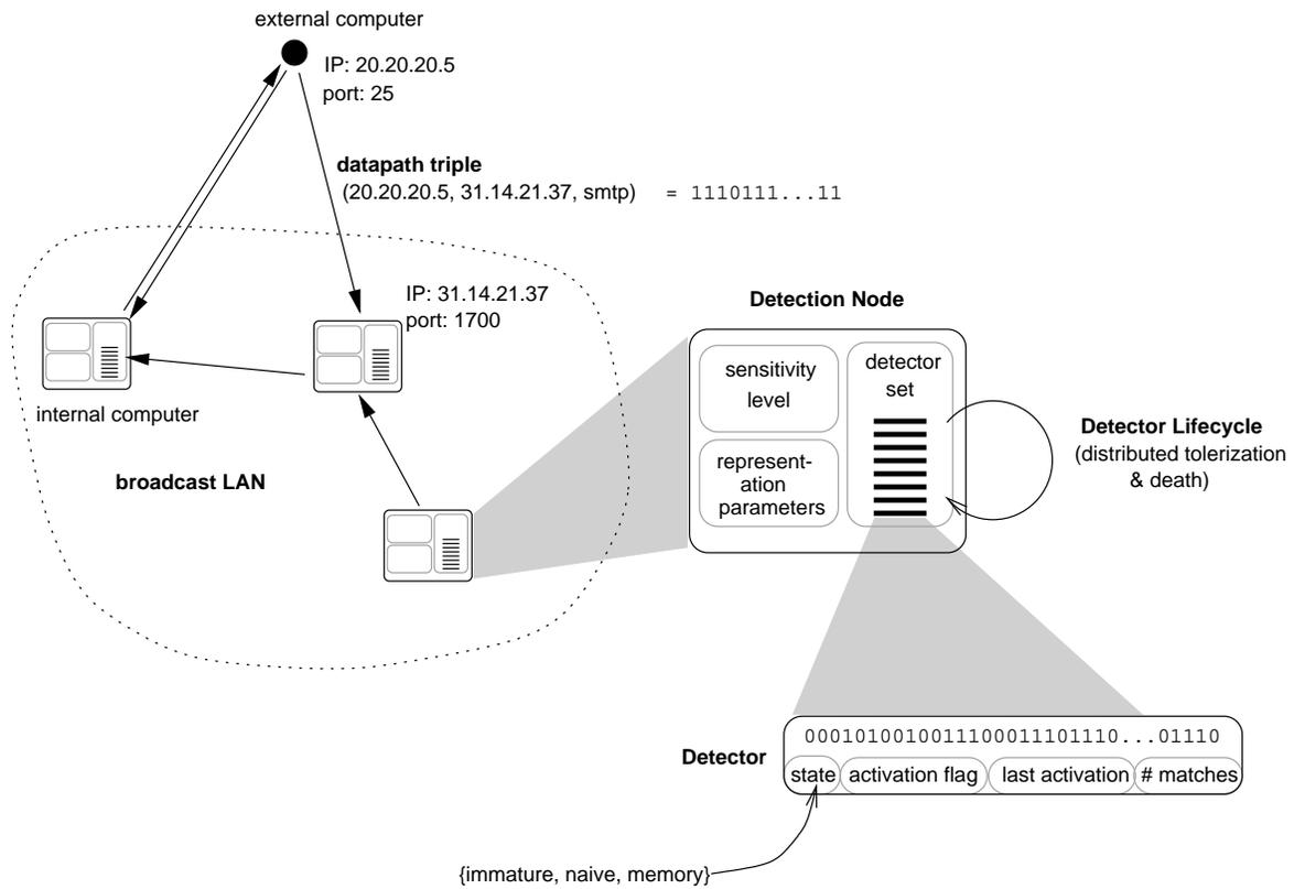
Figure 7: Architecture of LISYS. Each internal computer runs a detection node, which consists of a set of detectors, a local sensitivity level and a representation function with randomly generated parameters (for example, the permutation mask). Each detector contains a binary string, and is either immature, naive (and mature), or a memory detector. In addition, each detector keeps track of whether it is awaiting costimulation (using the activation flag) and how many matches it has accumulated.
