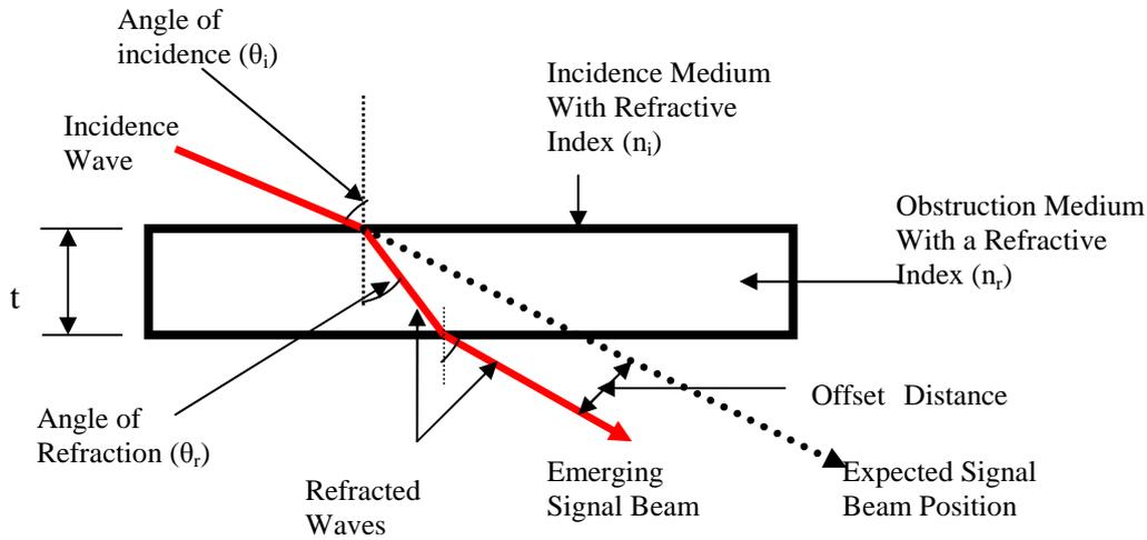
**Figure 1.** Signal Propagation Refraction Geometry [10]
