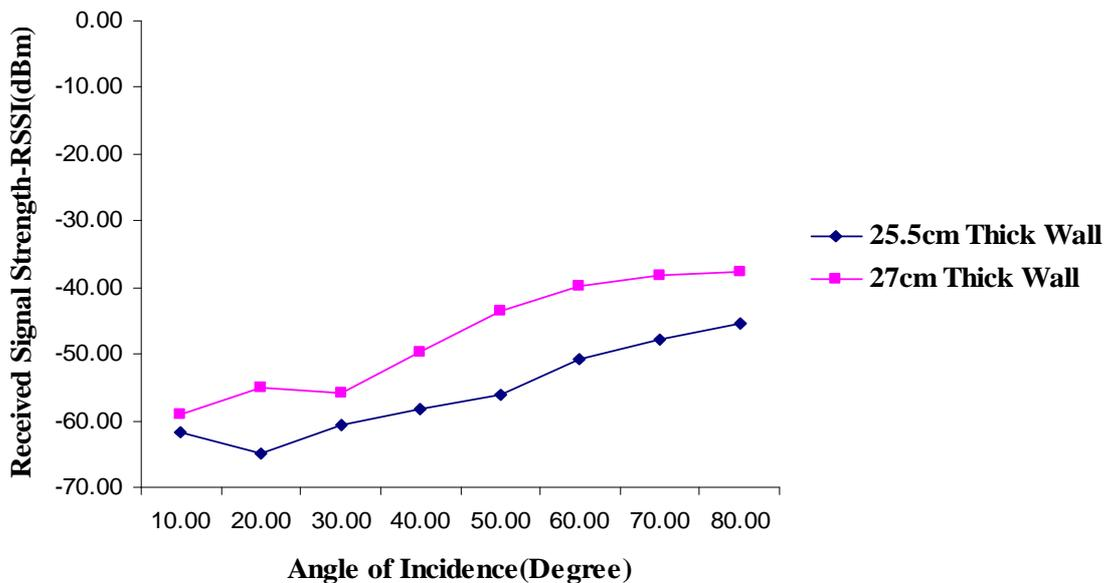
**Figure 4.** Effects of Angle of Incidence on Signal Strength through 25.5cm and 27 Thick Walls Test Site 2.
