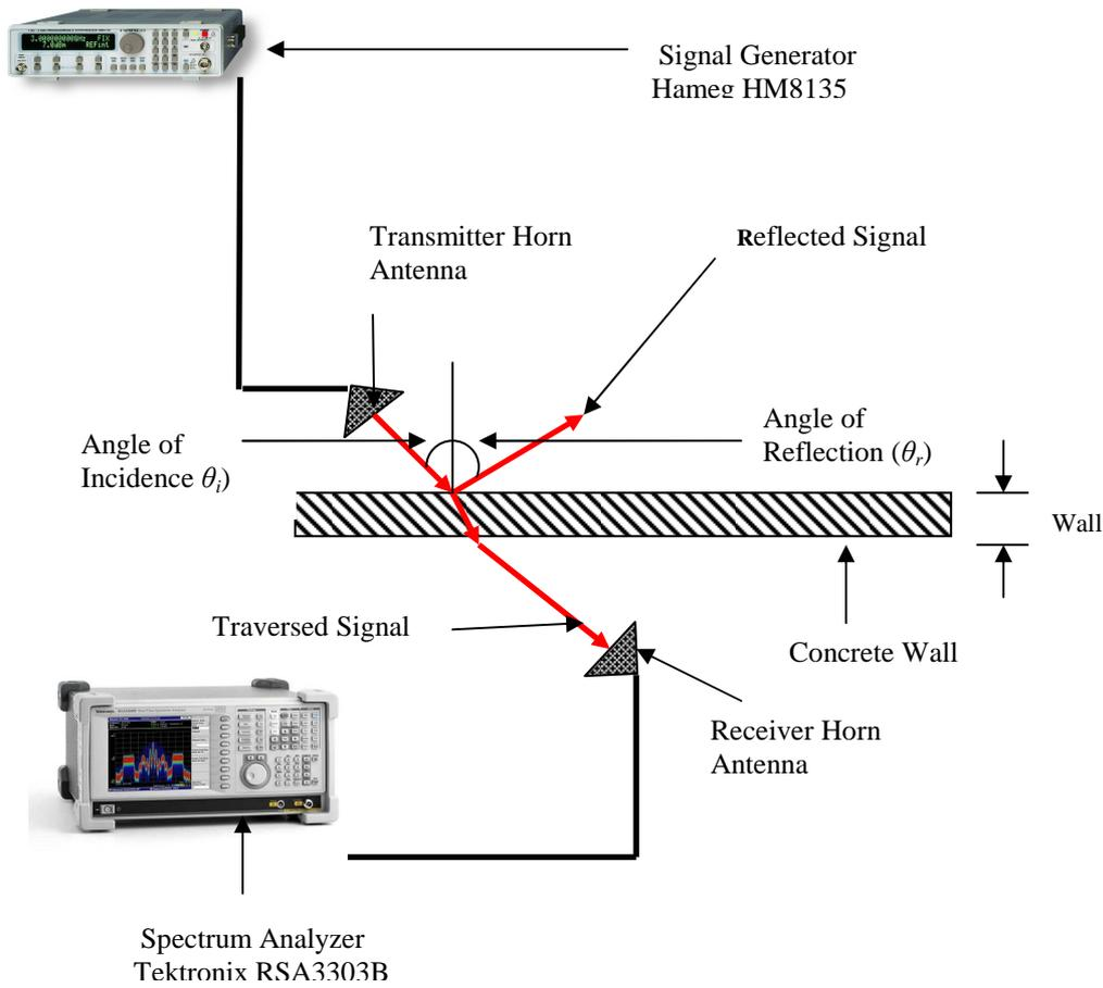
**Figure 2.** Experimental Setup for Angle of Incidence Tests
