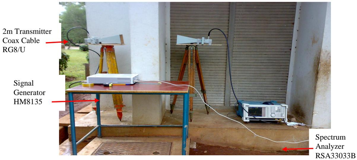
**Figure 1.** Signal Generator HM8135, Horn antennas and Spectrum Analyzer Tektronix RSA3303B Equipments Setup.
