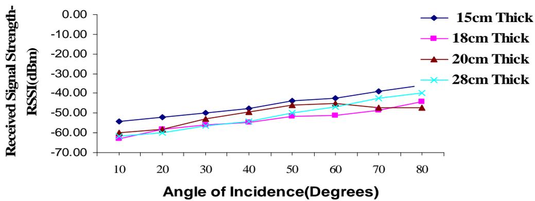
**Figure 3.** Effects of Angle of Incidence on Signal Strength through 15cm to 28cm Thick Walls in Test Site 1.
