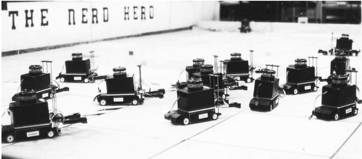
Figure 1: Some of the 20 mobile robots used to validate the group behavior methodologies we describe. These robots demonstrated group *safe-wandering*, *following*, *aggregation*, *dispersion*, *flocking*, and *foraging*.
