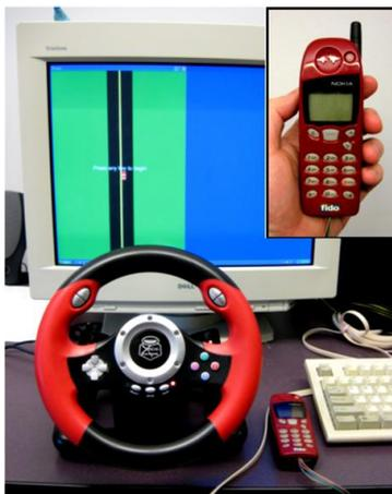
Fig. 1. Apparatus including the monitor, steering wheel, keyboard, and mobile phone. Inset: Close-up of the mobile phone used in the experiment.
