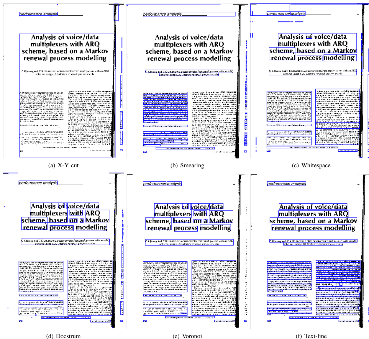
Fig. 7. Segmentation results from applying each algorithm to one page image. The page contains a title in large font and a big noise strip along the right border. (a) The x-y cut algorithm fails in the presence of noise and tends to take the whole page as one segment. (b) The smearing algorithm also classifies the detected regions as text/non-text, and thus misses the lines joined by the noise bar. (c),(d),(e) Due to the large font size and big inter-word spacing, the Voronoi, docstrum, and whitespace algorithms split the title lines. (f) Due to the noise bar, several characters on the right side of each line in the second column were merged with the noise bar and the text-line finding algorithm did not include these characters.
