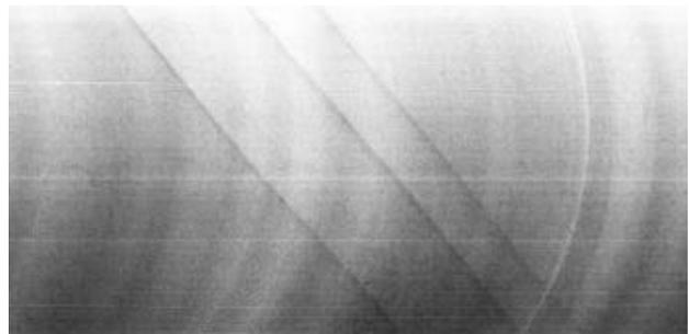
FIGURE 4. SHOCK WAVES 300 m ABOVE SR-71 AT M=1.25 AND 19.5 km RANGE
