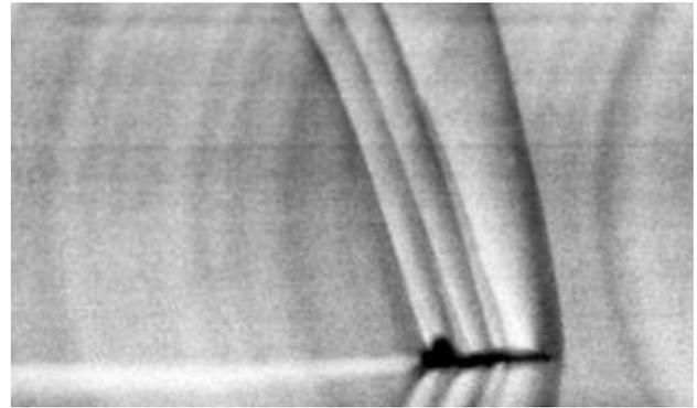
FIGURE 2. T-38 AT  $M=1.1$  AND 10 km RANGE
