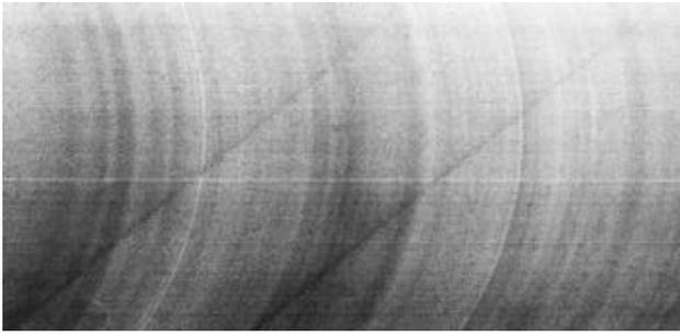
FIGURE 5. SHOCK WAVES 3.7 km BELOW SR-71 AT M=1.4 AND 19.5 km RANGE
