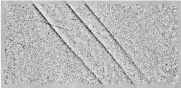
FIGURE 13. ENHANCED IMAGE OF SR-71 SHOCK WAVES FROM FIGURE 4
