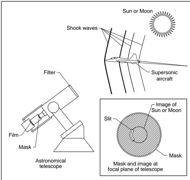
FIGURE 1. SETUP OF SCHLIEREN FOR AIRCRAFT IN FLIGHT
