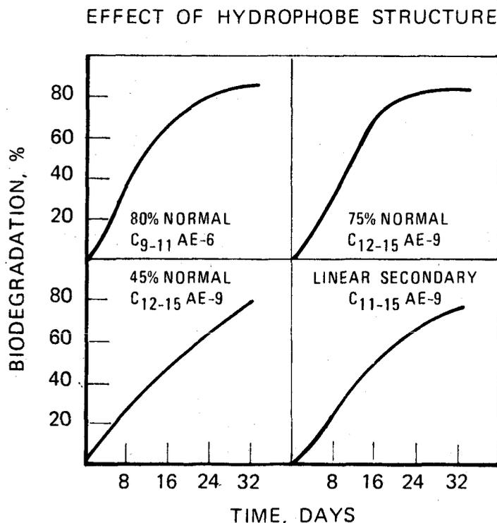
Figure 5/Ultimate biodegradation of AE
