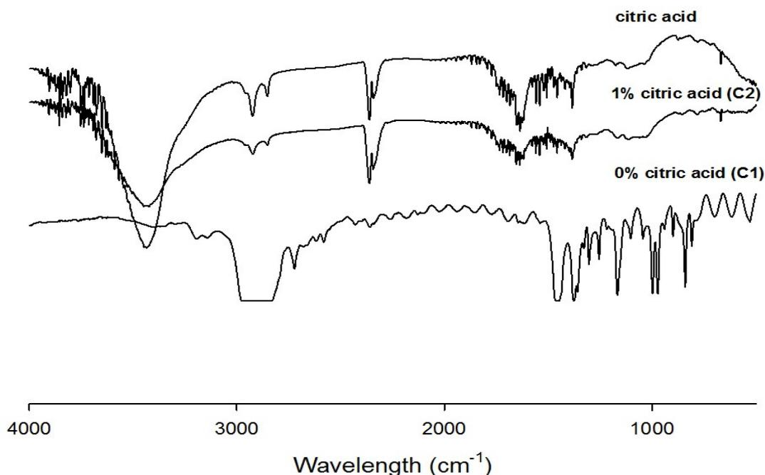
**Figure. 6. FTIR spectra of acid citric, dried coating polymer without (C1) and with (C2) citric acid.**
