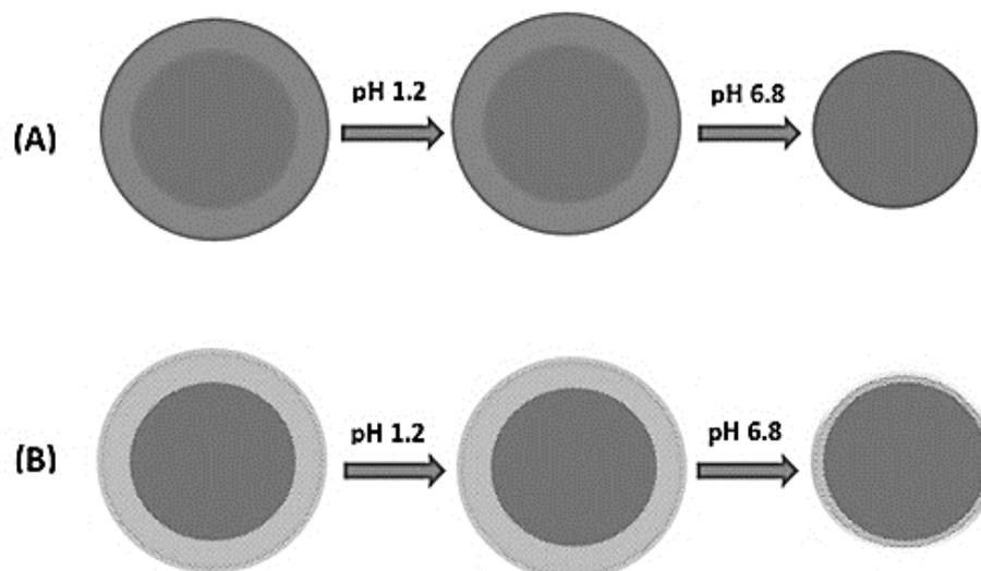
**Fig. 1. Schematic illustration of coated tablet in different pH conditions. (A) – without acidifier in coating polymer, (B) – acidifier in coating polymer.**
