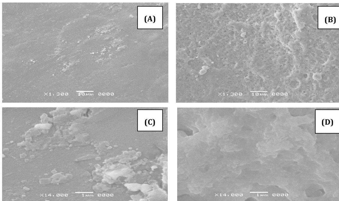
**Figure 7. SEM images of tablet without (A, C) and with (B, D) citric acid in coating polymer.**
