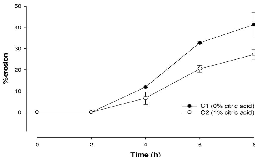
**Figure. 5. Erosion percent of tablet without (C1) and with (C2) citric acid in coating polymer after 2h at pH 1.2 and 4h, 6h, 8h at pH 6.8.**
