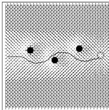
Figure 4: Reactive path generated via schema superpositioning.
