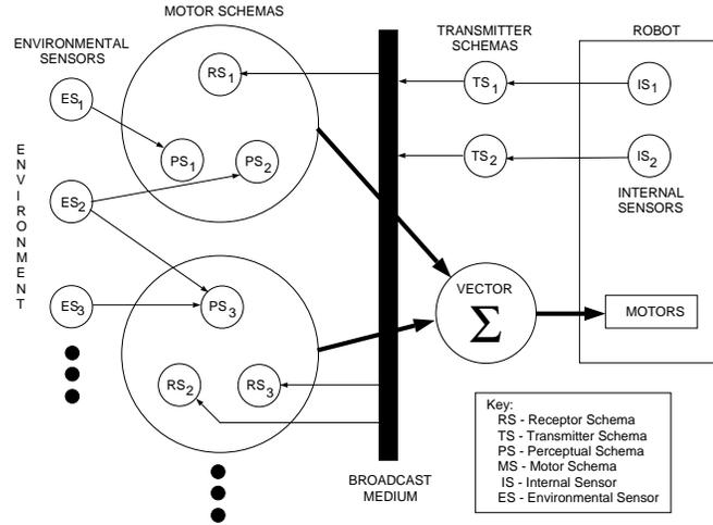
Figure 2: Process diagram for reactive component of AuRA
