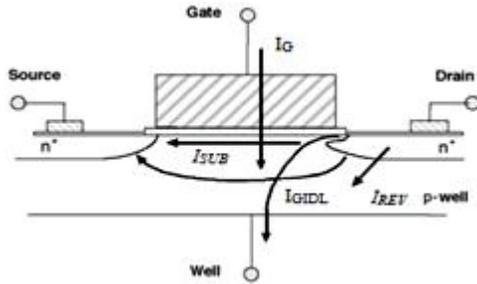
Figure2. Leakage current mechanisms of deep-submicron transistors.
