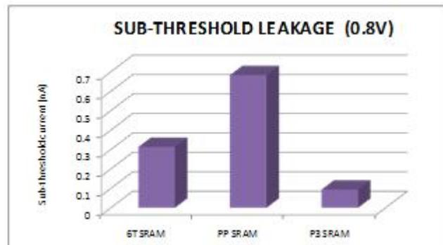
Figure 4. Sub-threshold Leakage Comparison at 0.8V
