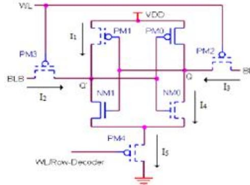
Figure3. P3 SRAM Sub-threshold Current Paths in Standby mode.
