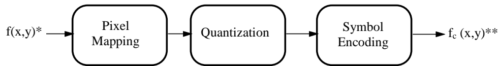
Fig. 2. Lossy compression model. * f(x,y) = original image; ** f_c(x,y) = compressed image.
