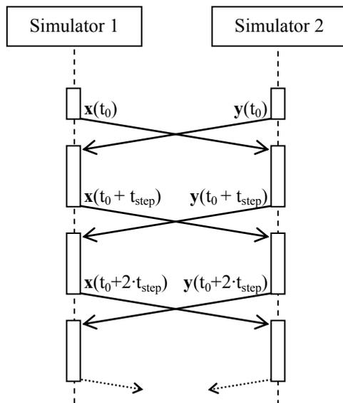
Figure 2. Co-simulation with fixed time step
