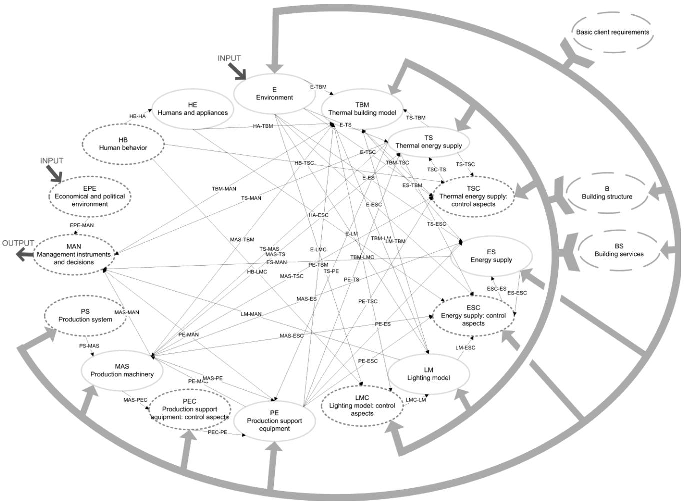
Figure 1. Generic production facility model (“Spider’s Web”)
