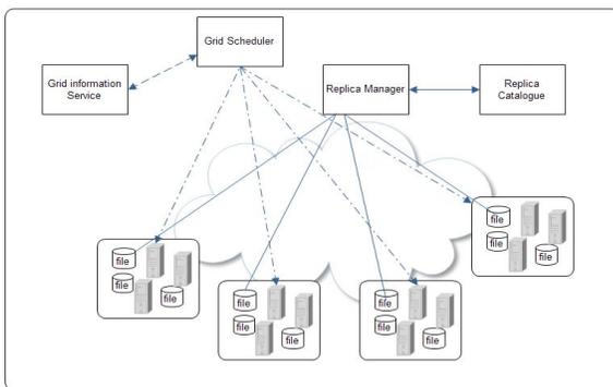
Figure 4: global model of centralized job scheduling and replication
