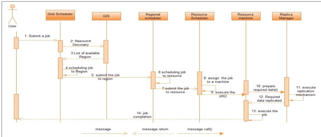
Figure 2: sequence Diagram of hierarchical job scheduling
