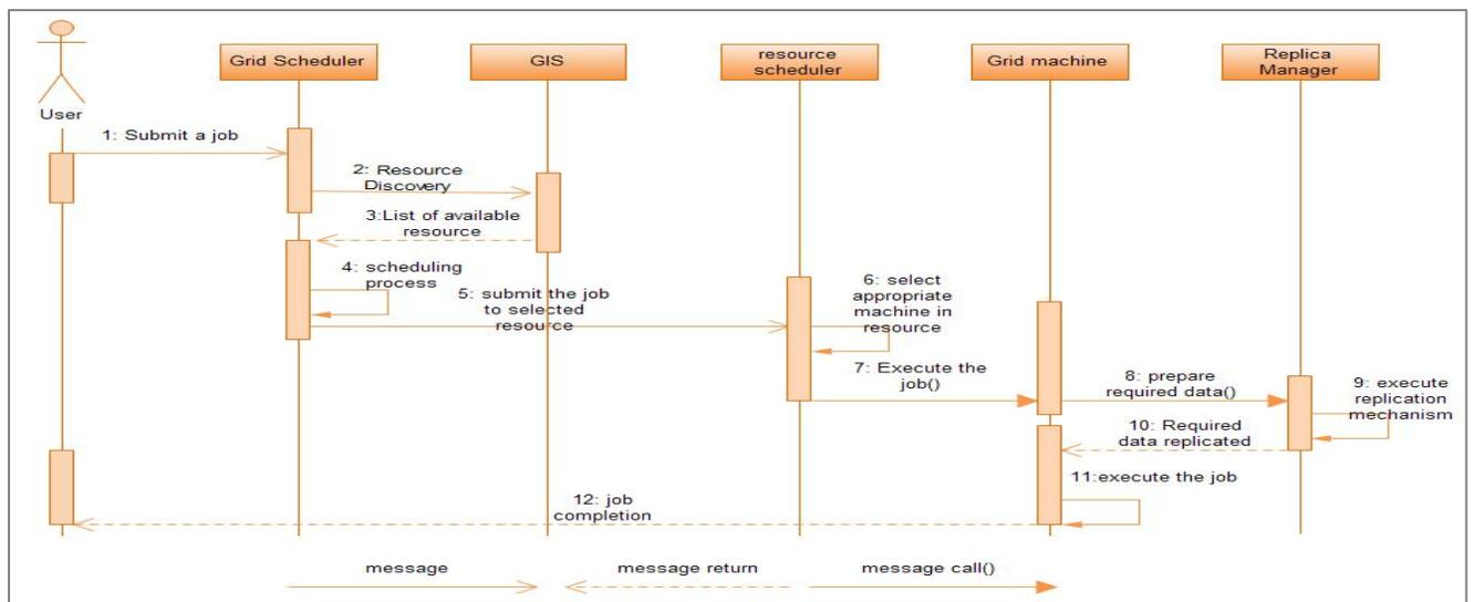
**Figure 1:** Sequence Diagram of centralized job scheduling
