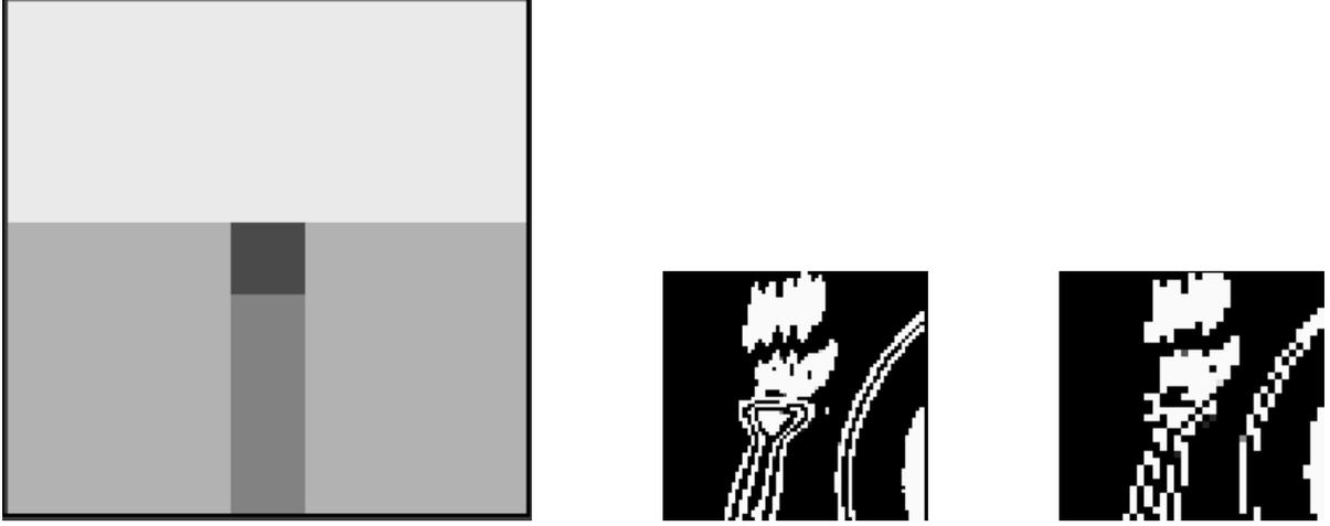
Figure 7: The left picture shows the shape of the Comet filter in greyscale (white corresponds to high values, black to low ones). The Comet filter shows high sensitivity (white areas) at ending contours and performs a robust orientation sensitive edge detection due to the “comet’s tail” (right pictures).
