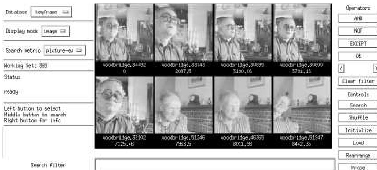
Fig. 9. An example of using appearance to sort keyframes from a video database; the sort is by general layout and color distribution.
