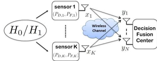
Fig. 1: The Decision Fusion model in presence of a (virtual) MIMO channel.
