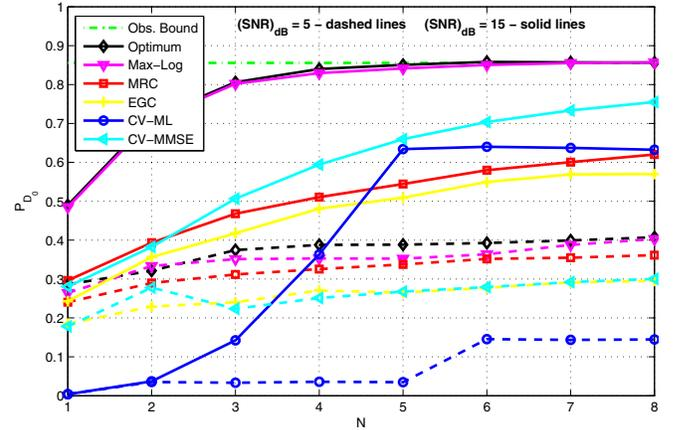
Fig. 5:  $P_{D_0}$  vs  $N$  for the presented rules;  $P_{F_0} \leq 0.01$ . WSN with  $K = 8$  sensors,  $(P_{D,k}, P_{F,k}) = (0.5, 0.05)$ ,  $k \in \mathcal{K}$ .  $(SNR)_{dB} \in \{5, 15\}$ .
