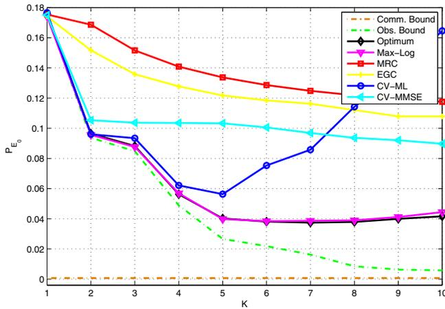
Fig. 7:  $P_{E_0}$  vs  $K$  for all the rules presented; WSN with  $N = 2$  antennas at DFC and channel  $(SNR)_{dB} = 15$ ;  $(P_{D,k}, P_{F,k}) = (0.7, 0.05)$ ,  $k \in \mathcal{K}$ .
