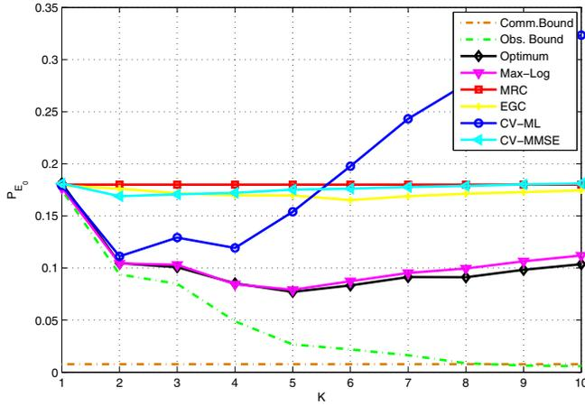
Fig. 6:  $P_{E_0}$  vs  $K$  for all the rules presented; WSN with  $N = 1$  antenna at DFC and channel  $(SNR)_{dB} = 15$ ;  $(P_{D,k}, P_{F,k}) = (0.7, 0.05)$ ,  $k \in \mathcal{K}$ .
