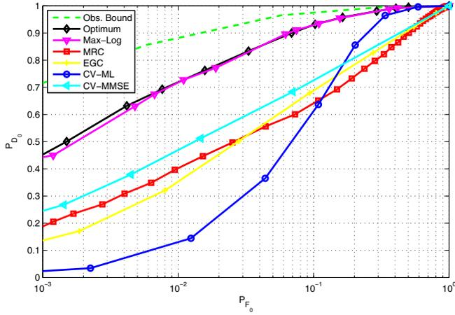
Fig. 3: ROC for the presented rules. WSN with  $K = 8$  sensors,  $(P_{D,k}, P_{F,k}) = (0.5, 0.05)$ ,  $k \in \mathcal{K}$ .  $N = 2$ ,  $(SNR)_{dB} = 15$ .
