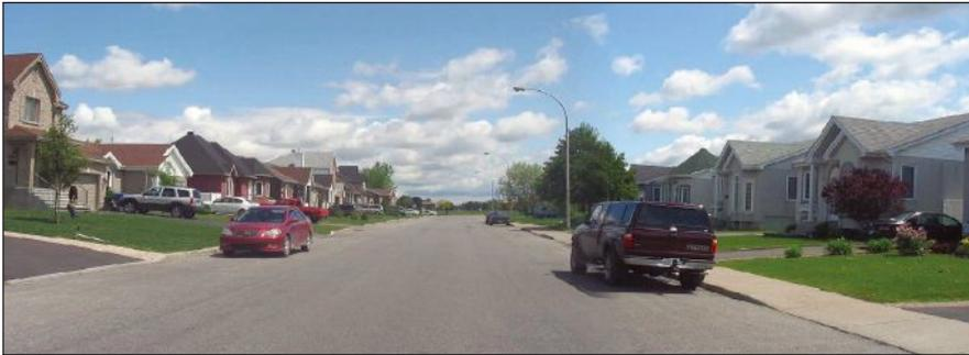
Figure 2. Example of a road with a credible limit of 31 mph (50 km/h)
