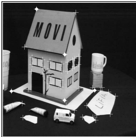
Figure 5.3: The house scene: the three images used for reconstruction together with the extracted corners. The reference frame used for the reconstruction is defined by the five points marked with white disks in image 3
