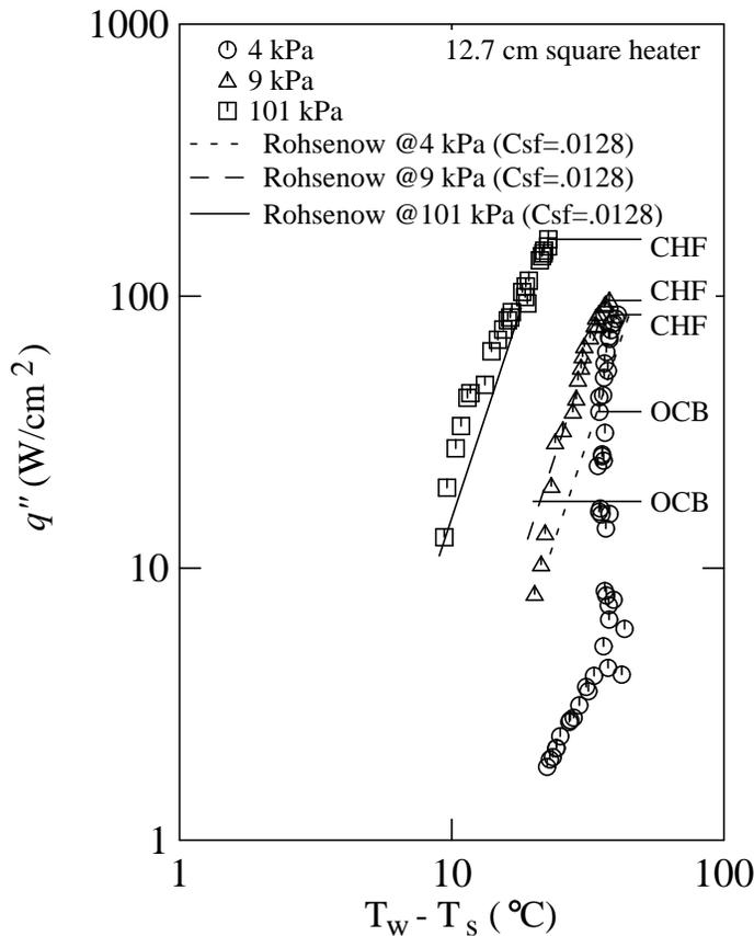
**Figure 7:** Nucleate boiling curves for water on a 1.27 cm square copper heated surface with an emery paper finish. Pressures were maintained at 4, 9, and 101 kPa. Rohsenow correlation plotted for comparison.
