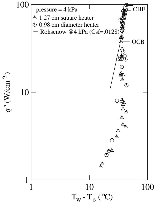
**Figure 8:** Effect of heater size on nucleate boiling. The measured CHF condition and the onset to continuous boiling predicted by equation (6) are indicated. Rohsenow correlation plotted for comparison.
