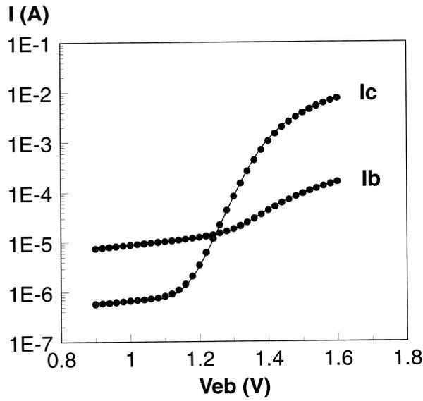
Figure 11.9 Gummel plot dc characteristics of GaAs HBT.
