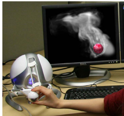
Fig. 1. The user grasps the handle of the Novint Falcon to move the spherical object and feel the forces it experiences in the fluid.
