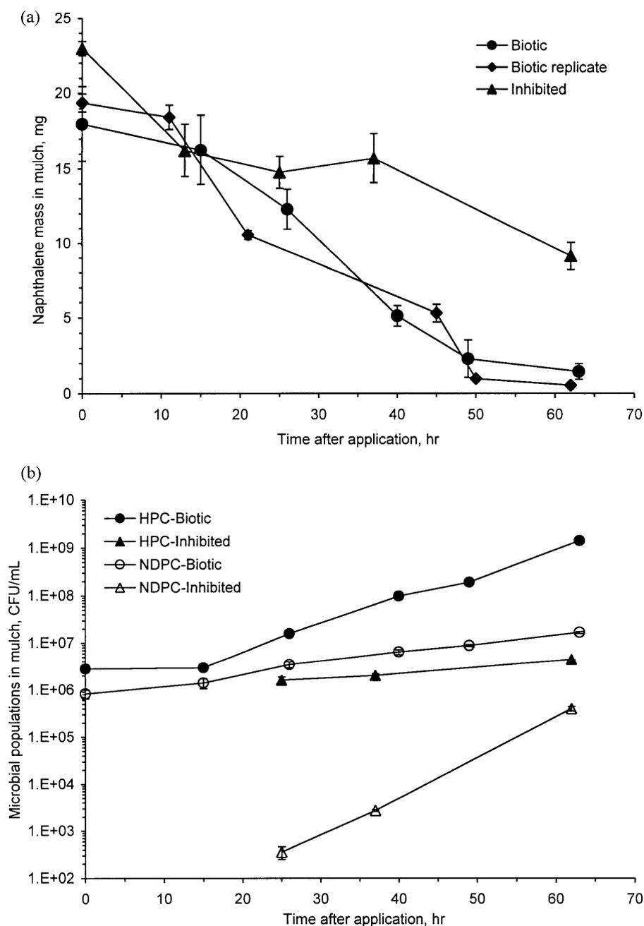
**Figure 3—Phase 2 results for the dissolved naphthalene experiments: (a) Average mass of naphthalene in the mulch of the biotic, biotic replicate, and inhibited-control reactors; and (b) average total heterotrophic plate counts (HPC) and naphthalene-degrader plate counts (NDPC) in the mulch of the biotic and inhibited-control reactors (biotic replicate data not shown for clarity). Error bars represent  $\pm$  one standard deviation.**
