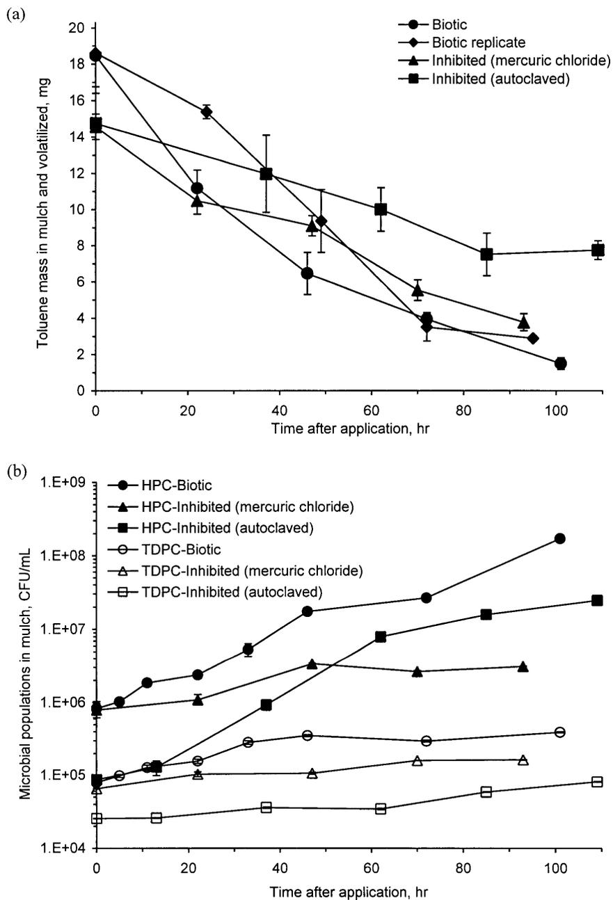
**Figure 5—Phase 2 results for the dissolved toluene experiments: (a) Average mass of toluene in the mulch and activated carbon of the biotic, biotic replicate, and inhibited-control reactors, and (b) average total heterotrophic plate counts (HPC) and toluene-degrader plate counts (TDPC) in the mulch of the biotic and inhibited-control reactors (biotic replicate data not shown for clarity). Error bars represent  $\pm$  one standard deviation.**
