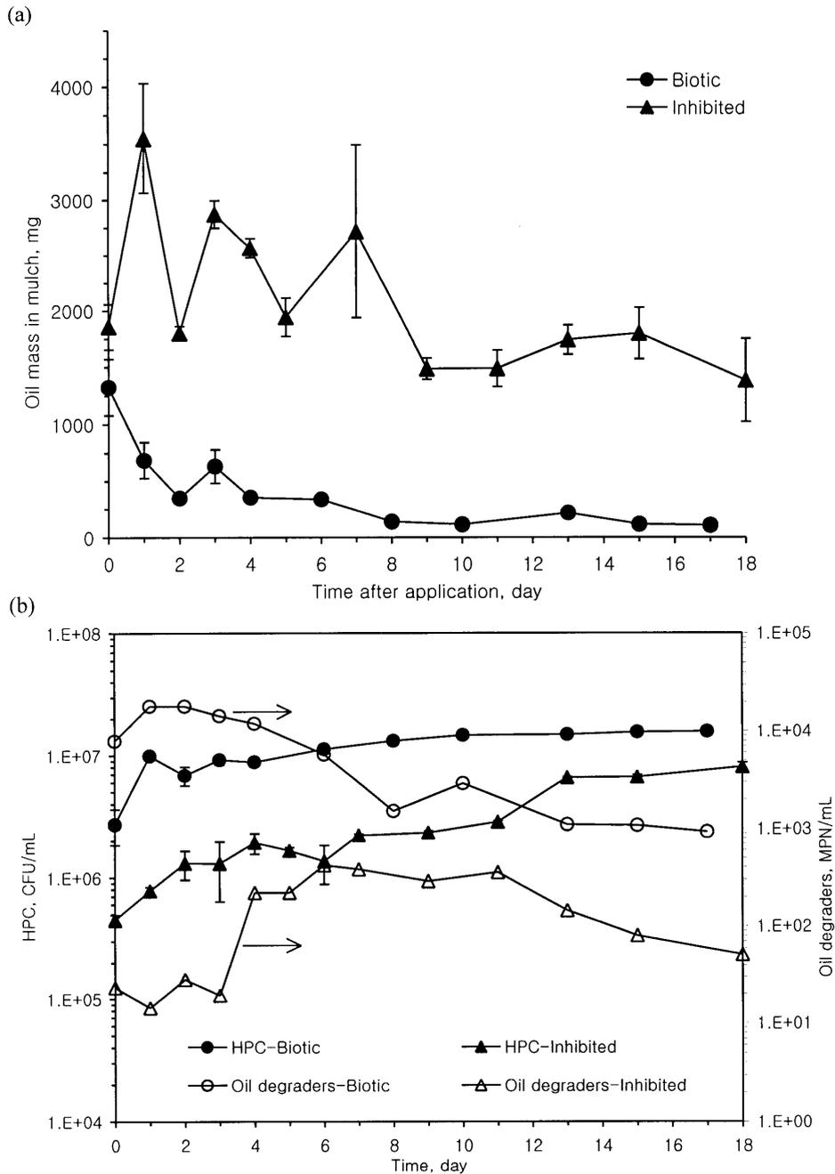
**Figure 7—Phase 2 results for the motor oil experiments: (a) Average mass of oil in the mulch; and (b) average total heterotrophic plate counts (HPC) and oil-degrader counts (MPN) in the mulch. Error bars represent ± one standard deviation.**
