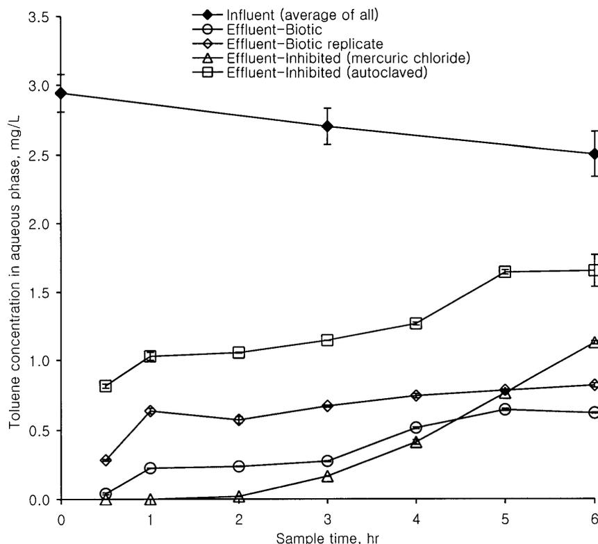
**Figure 4—Influent and effluent average toluene concentrations in the aqueous phase during the Phase 1 simulated storm event in the biotic, biotic replicate, and inhibited-control reactors. Error bars represent  $\pm$  one standard deviation.**
