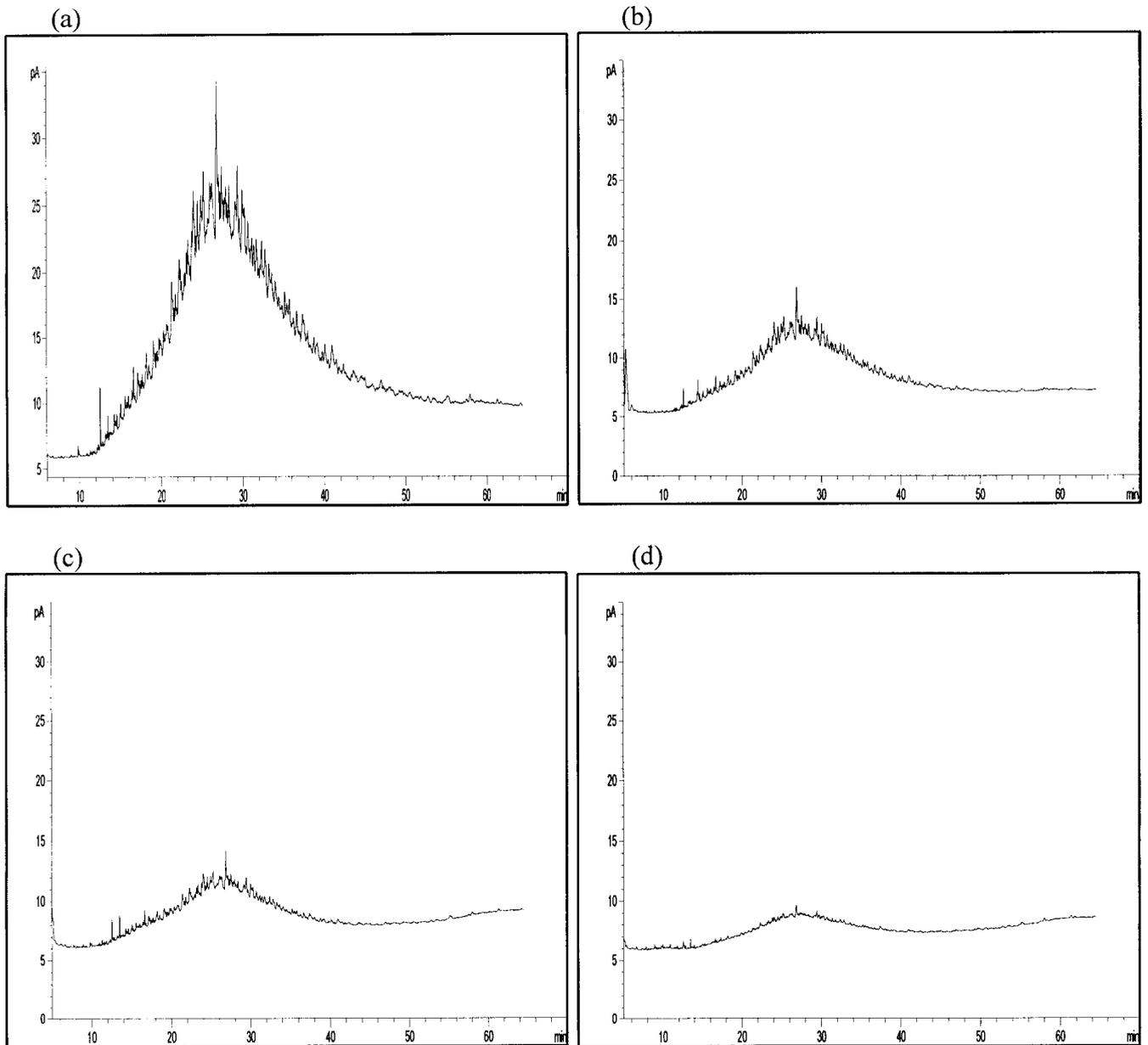
**Figure 6—Representative gas chromatograms of oil extracted from the mulch during Phase 2 in the biotic experiment at times (a) 0, (b) 2, (c) 3, and (d) 10 days, and in the inhibited-control experiment at times (e) 0, (f) 5, and (g) 11 days.**
