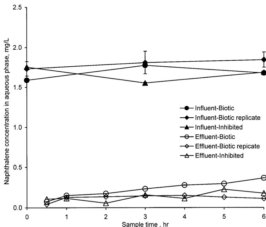
**Figure 2—Influent and effluent average naphthalene concentrations in the aqueous phase during the Phase 1 simulated storm event in the biotic, biotic replicate, and inhibited-control reactors. Error bars represent ± one standard deviation.**
