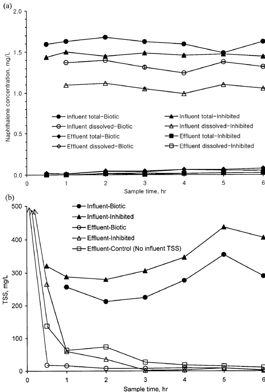
**Figure 8—Naphthalene and total suspended solids (TSS) data for the aqueous phase during the Phase 1 simulated storm events in the particulate-associated naphthalene experiments: (a) Influent and effluent average total and dissolved naphthalene concentrations, and (b) influent and effluent TSS concentrations. Initial effluent TSS values (at t = 0) exceeded 1000 mg/L and are not shown. Error bars represent ± one standard deviation.**
