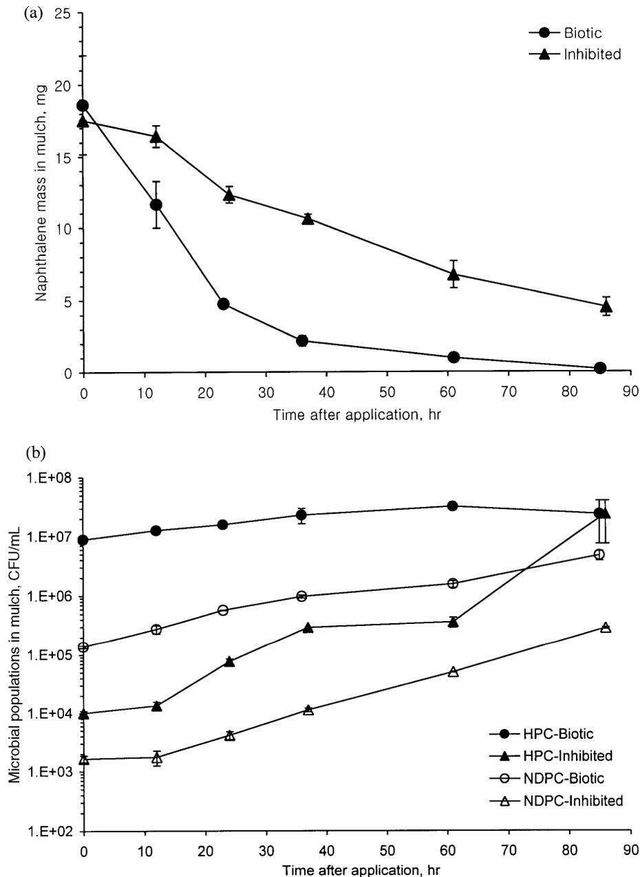
**Figure 9—Phase 2 results for the particulate-associated naphthalene experiments: (a) Average mass of naphthalene in the mulch; and (b) average total heterotrophic plate counts (HPC) and naphthalene-degrader plate counts (NDPC) in the mulch. Error bars represent  $\pm$  one standard deviation.**
