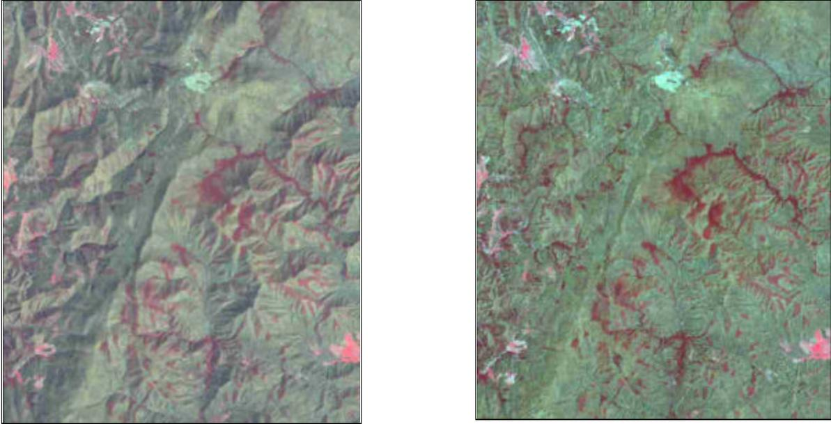
**Figure 1.** Examples results of 1984 satellite image atmospheric correction and topographic normalization in Shenandoah National Park, before (left) and after (right). Notice reduction in shadows and haze.
