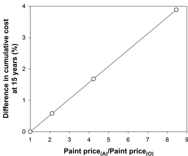
Figure 5. Effect of paint price on cumulative operating costs over 15 years. Variation in paint price is expressed as a multiple of the standard price of the fouling-control topcoat [Paint price (O) ]. Change in cumulative operating costs is expressed as a percentage of the cumulative costs assuming the standard topcoat price.
