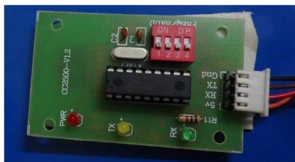
**Figure 5: PIC Microcontroller in Transmitter Section**
