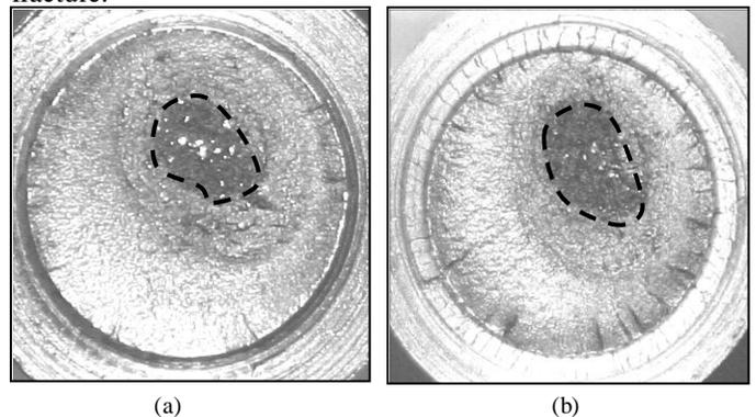
Fig 5. Micrographs of fatigue fracture surface at stress amplitude of 120MPa for (a)  $Ra = 1.778\mu\text{m}$  and (b)  $Ra = 5.484\mu\text{m}$ .
