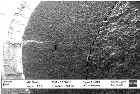
Fig. 6. SEM micrograph of different region of fracture surface
