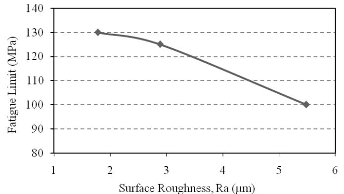
Fig. 4. Summary of fatigue limits of analyzed specimens.
