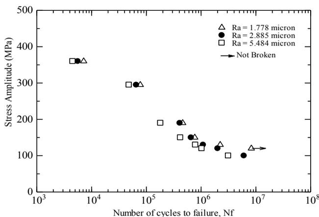
Fig. 3. S-N curve for different surface roughness
