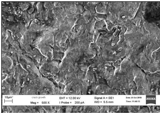
Fig. 7. SEM micrograph of fatigue fracture surface for stable crack propagation region
