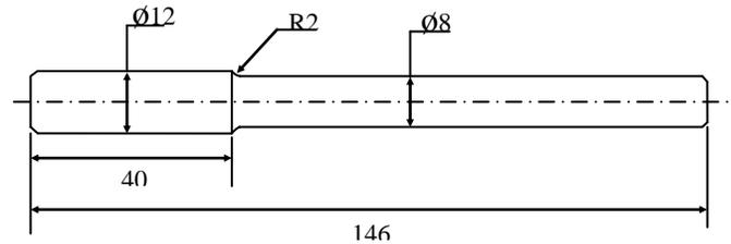
Fig. 1. Detail dimension of fatigue specimens (mm)
