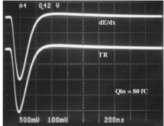
Figure 8. Impulse response of the P/S.
