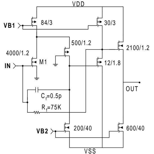
Figure 4. Current sensitive preamplifier.
