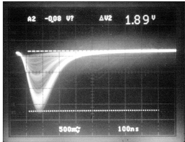
Figure 9. Response to  $^{55}\text{Fe}$  X-ray photons.
