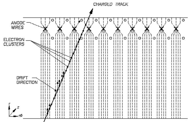
Figure 2. Time Expansion Chamber showing anode/cathode configuration, electric field lines and drift direction of electron clusters created by ionizing particles.
