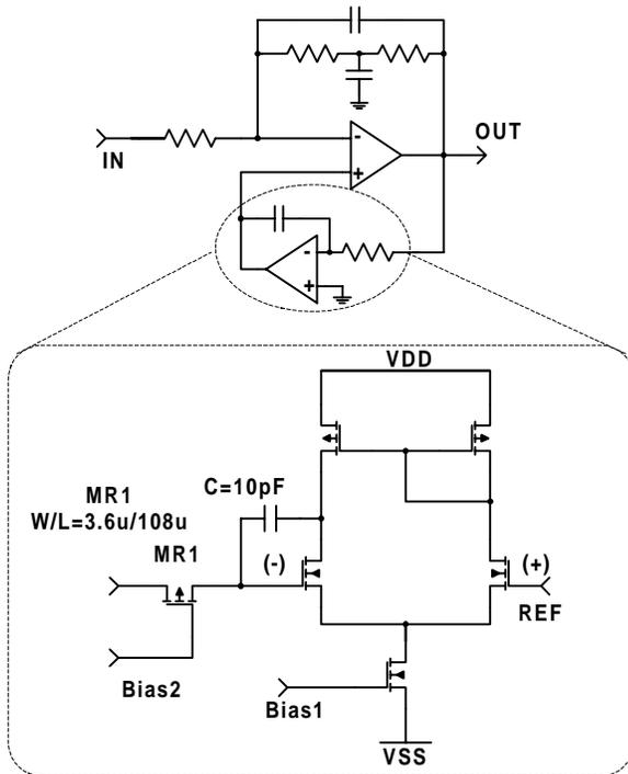
Figure 5. AC coupling by an integrator in feedback.
