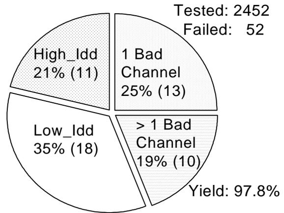
Figure 11. Failure modes.
