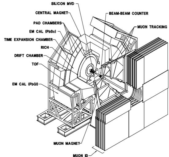
Figure 1. PHENIX detector.
