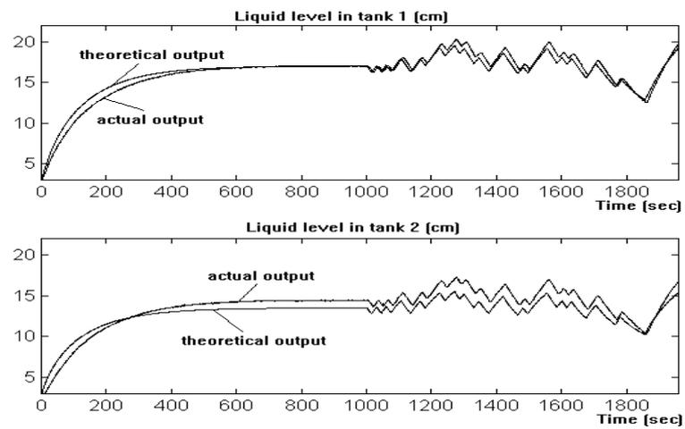
Fig. 2 Theoretical outputs of the model and actual outputs of the physical system.
