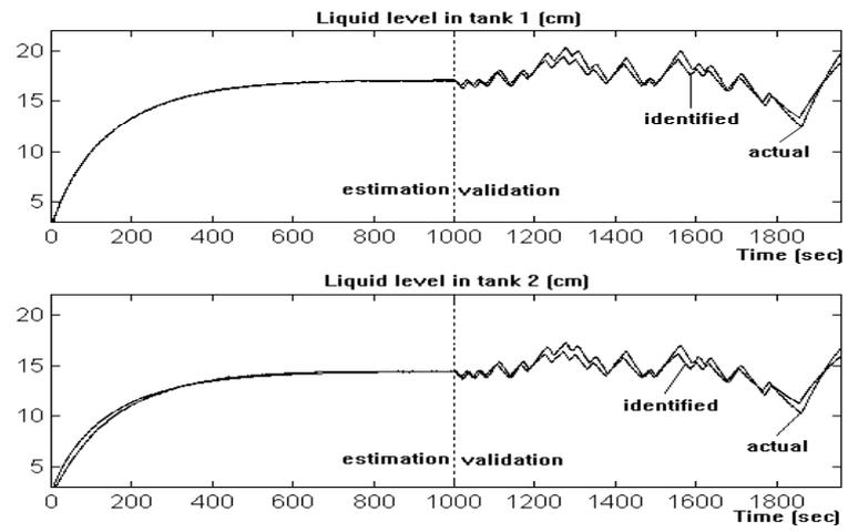
Fig. 5 Outputs of the identified model and actual outputs of the physical system.
