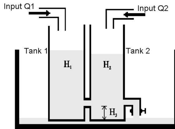
Fig. 1 A nonlinear coupled liquid-level regulation system.
